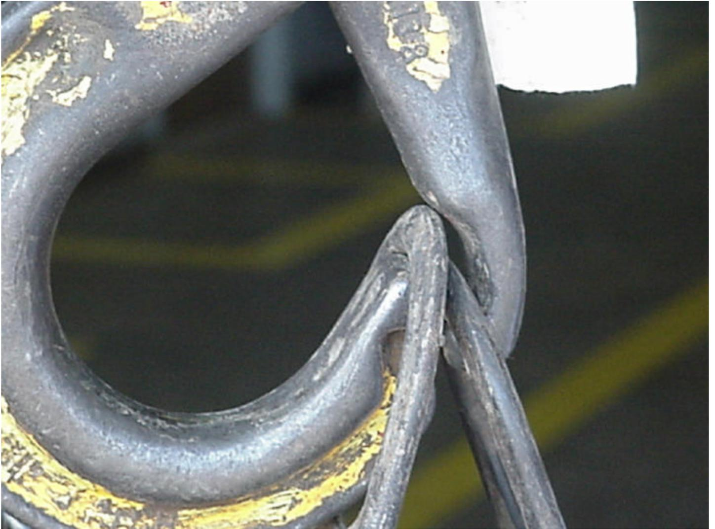
Photograph of "D" Rings in Hook/Latch Gap
