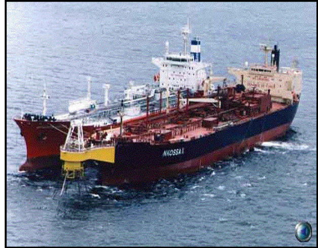
Figure 6.9: NKOSSA II equipped with side-by-side system. Courtesy of Navion.
