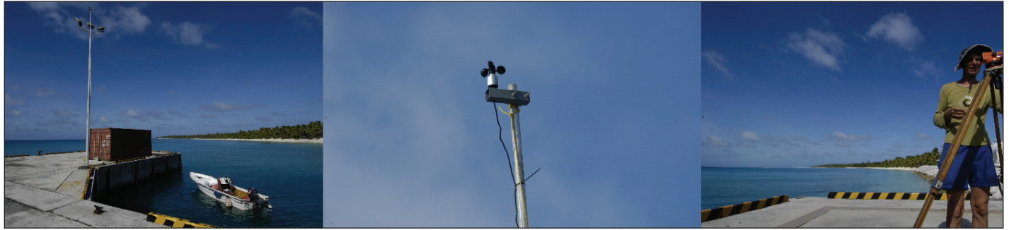
Figure 12.18. Measurement of physical data: drifting across reef flats with instruments in a dry-bag (left), wind speed logging (center) and land height surveying (right). Photos: A Seale.
