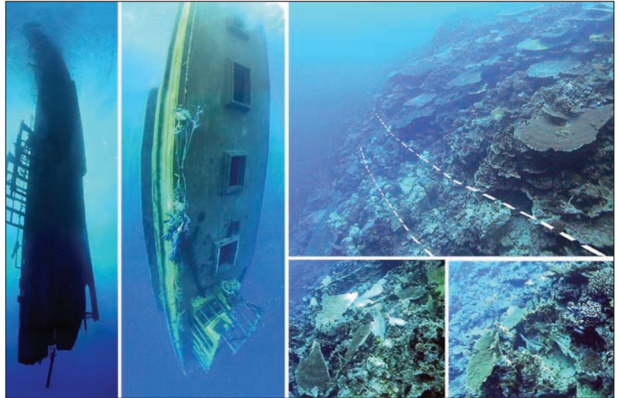
Figure 12.11. In 2006 an abandoned, partially sunk wooden boat (resembling an Indonesian fishing vessel) resulted in several days of reef damage along the dropoff, as the currents moved the wreck back and forth along the central southern shore of Majuro atoll. Photos: D. Jacobson.
