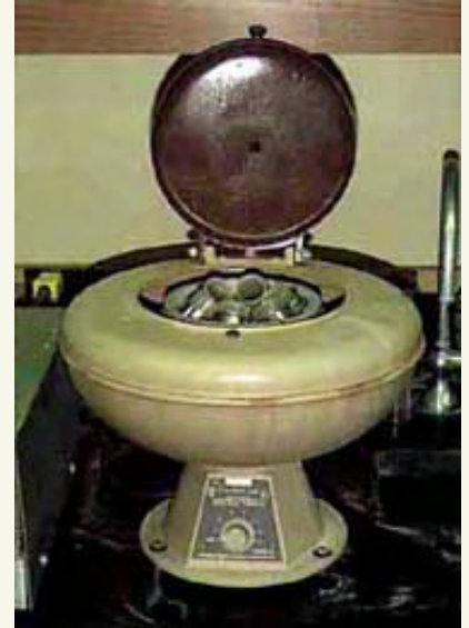
A centrifuge used to "spin down" materials.
