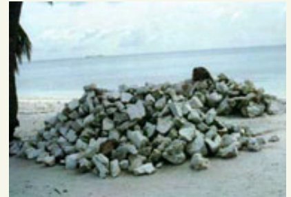
Coral stones and blocks have been used for house construction in many parts of the tropical world. (Photo: Bluepeace/Maldives)
