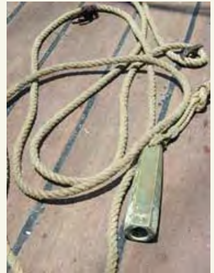
A lead line on the deck of a ship (Photo: Ocean Institute)
