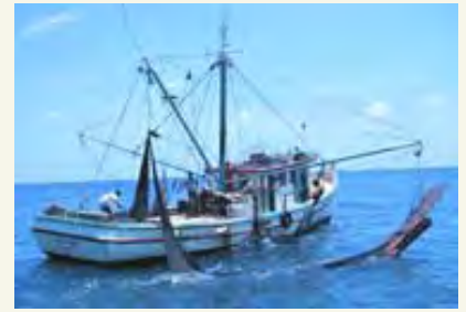
a double-rigged shrimp trawler with bag of one net on board (Photo: NOAA)
