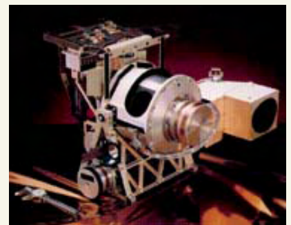
This SeaWiFS (Sea-viewing Wide Field-of-view Sensor) is an ocean color sensor.
