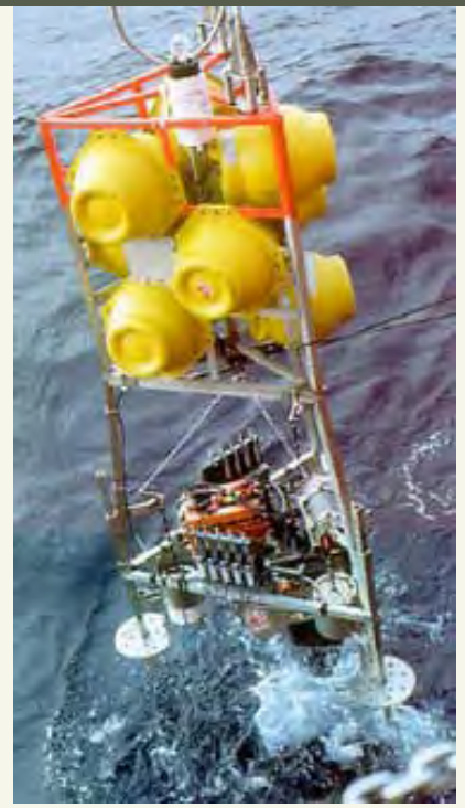
A lander system being deployed. The part with the large yellow structures is the floatation rack (Photo: KC Denmark)
