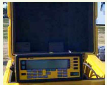
Portable GPS unit utilized in surveying.
