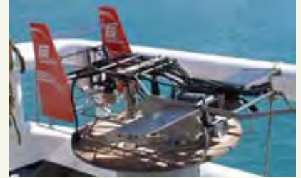
A towed optical assessment (TOAD) device is used to record bottom characteristics (Photo: NOAA)
