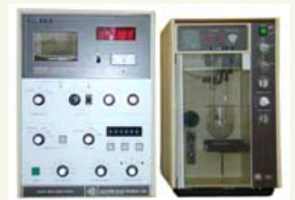
A Coulter counter is an instrument used to measure the distribution of particle size.
