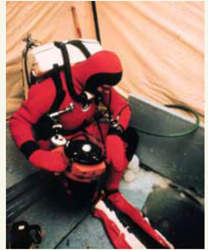
Arctic diver with rebreather and heated dry suit prepares to descend into the ice. (Photo: NOAA/OAR/National Undersea Research Program)
