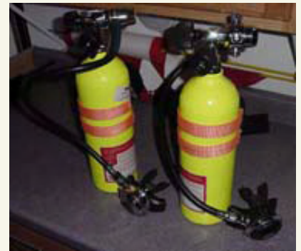
The first stage regulator is attached to the scuba tank. (Photo: NOAA/ National Undersea Research Program)
