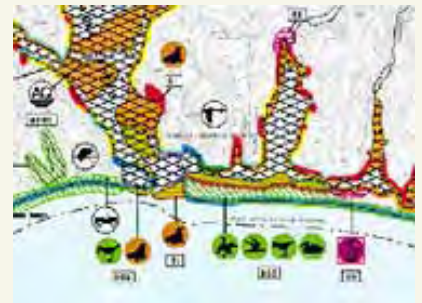
A section of an Environmental Sensitivity Index map, showing part of the Point Reyes National Seashore. Shorelines are color-coded to show their sensitivity to oiling. (Photo: NOAA)
