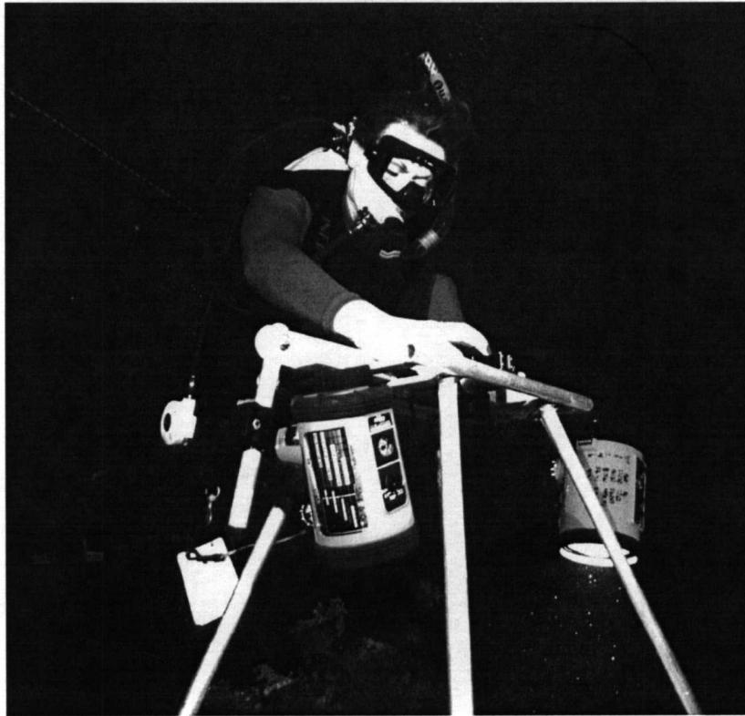
Figure 2.3.0.1. Diver with random transect camera framer.
