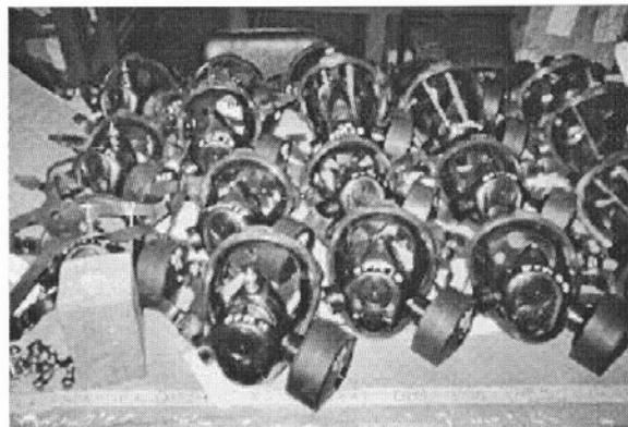
Figure 13, Probed and Un-probed Respirators During the Course of Preparing for LRPL Testing
