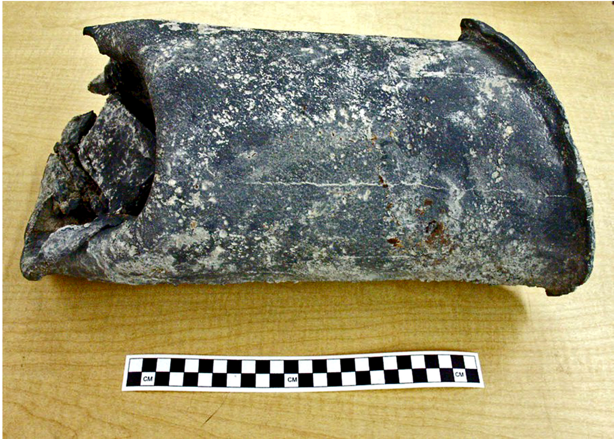
Figure 16. Interior opening of conserved lead hawse pipe from the Mica shipwreck. Note the possible cut marks on the curled-in exterior surface, visible in the lower left (Photograph by Dave Ball).
