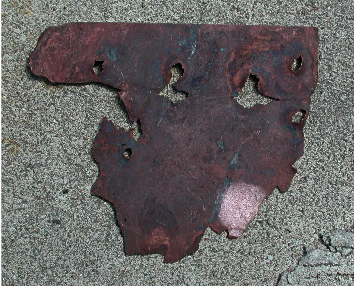
Figure 17. A fragment of the copper sheathing retrieved from the Mica shipwreck. The bright spot in the lower right corner has been mechanically cleaned with a glass bristle brush (Photograph by Toby Jones).
