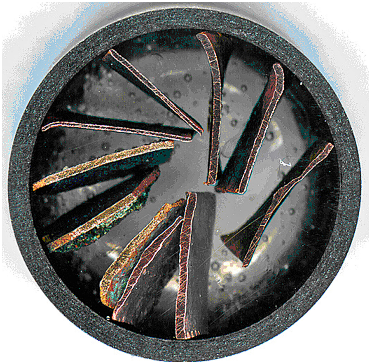
Figure 14. The refracting electron microprobe sample carrier. It contains pieces of metallic sheathing awaiting analysis (Photograph courtesy of Dr. Renald Guillemette).
