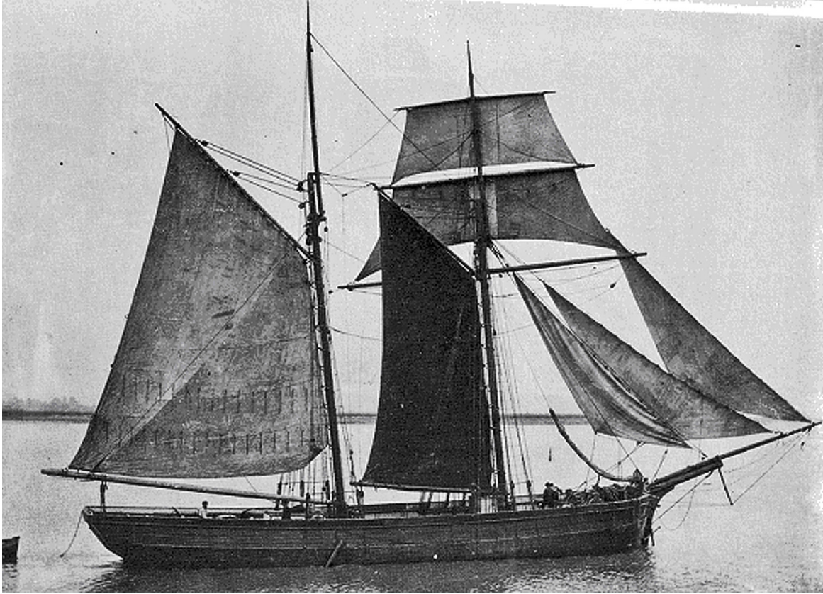
Figure D3. The two-masted fore-and-aft rigged merchant schooner Hope . The vessel is shown with double topsails and no studding sail (From MacGregor 1997: 67).
