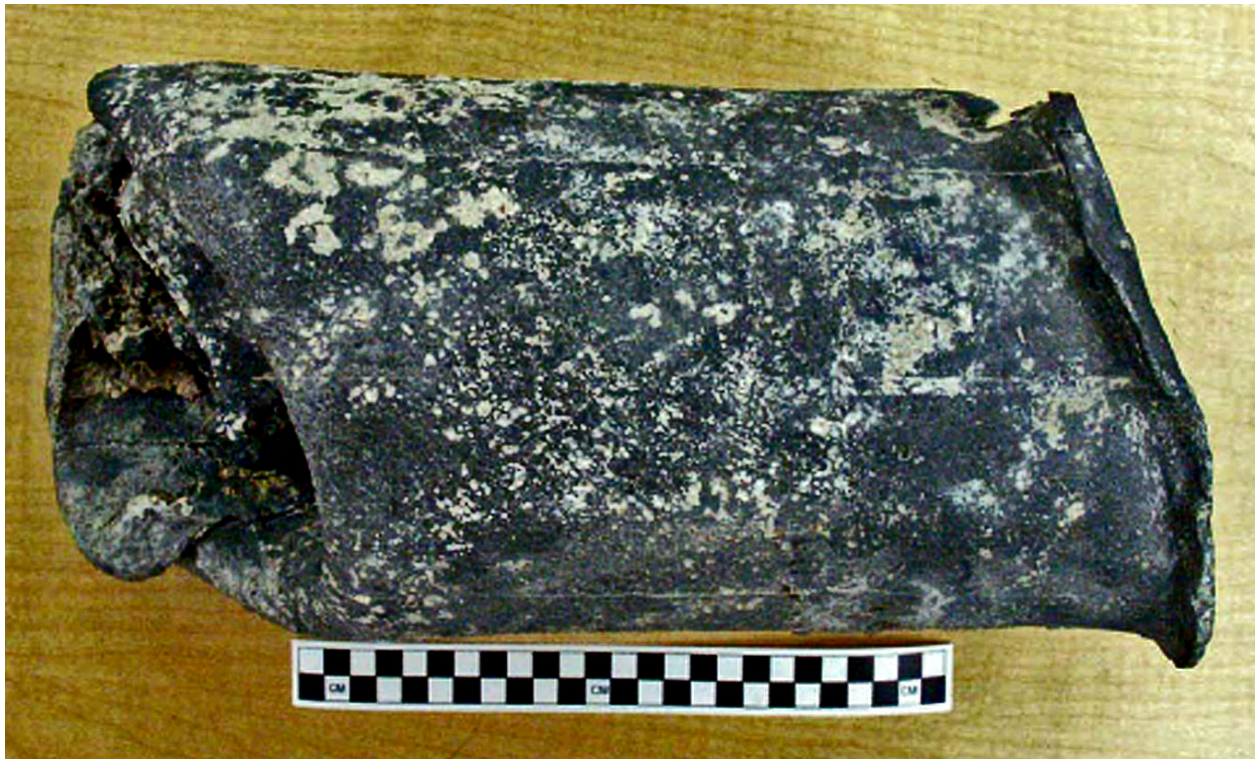
Figure 15. Forward face of lead hawse pipe from the Mica shipwreck. Casting seams are evident on the both the external (right) and internal (left) openings (Photograph by Dave Ball).
