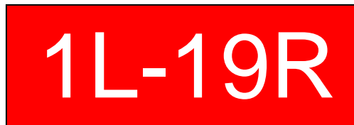
Runway Hold Sign
