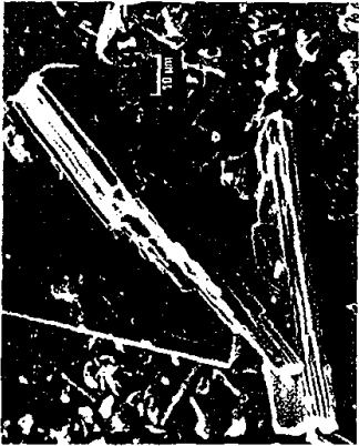
FIGURE 24. - Riebeckite, showing prismatic shape (SEM photomicrograph at X 800).
