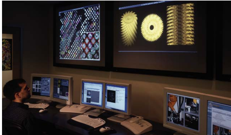
■ Researchers set up and monitor their cryo-electron microscopy experiments from this state-of-the-art control room at NRAMM. The large screens display images acquired by the microscope as well as results of image analysis and processing.
