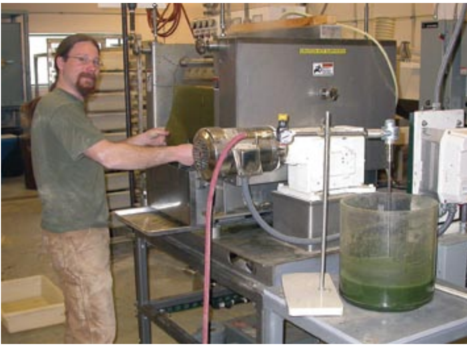
Lucas Porter, University of Idaho student, manufactures flake feeds at the Bozeman Fish Technology Center with a drum dryer for endangered Rio Grande silvery minnow propagation. Experimental feeds are provided by U.S.D.A. fish nutritionist Dr. Rick Barrows for use by facilities in New Mexico.
