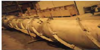
Pipe with Helical strakes
