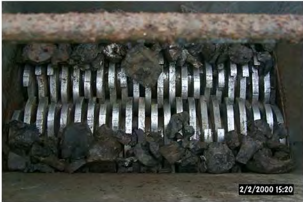
Fig. 6 - SubSea Rock Crushing Assembly Used in SubSea MudLift JIP 1
