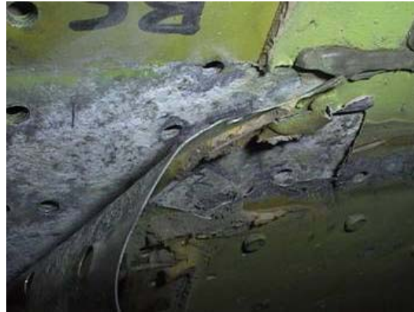
corrosion of a KC-135 lap joint region
