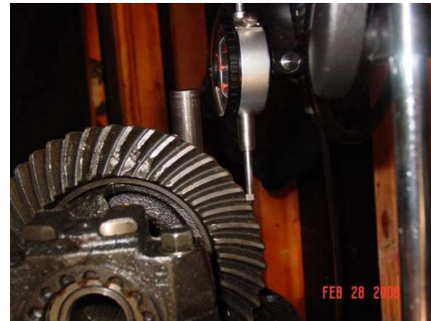
Wear initiates backlash impacts (stiffness discontinuity)
