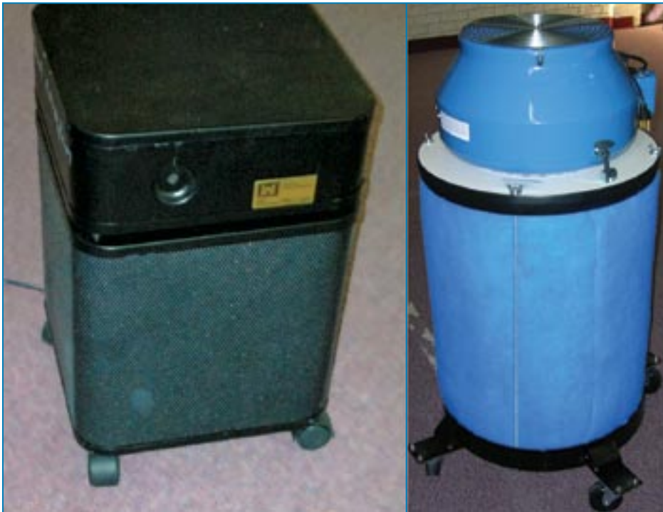
Figure 4-5: Two recirculation filter units.
