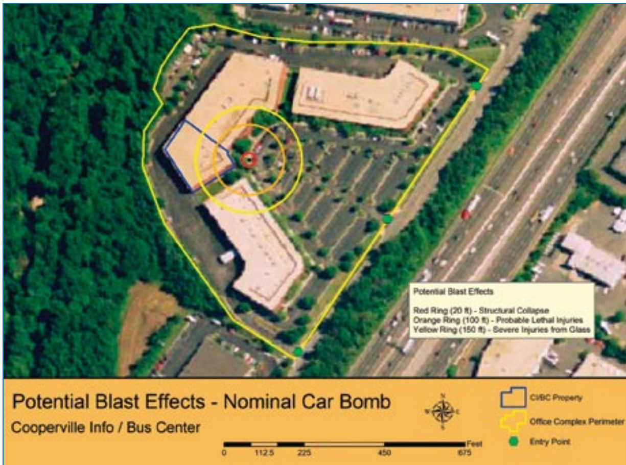
Figure 5-3: Blast effects related to access control.
