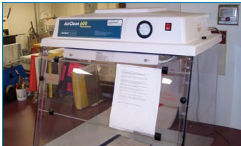
Figure 5-6: Example of an air sampling system in a mailroom.
