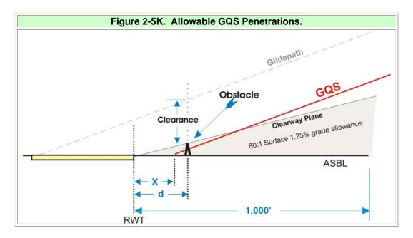
Additionally, frangible radar reflectors and other objects required for Category I/II/III instrument landing operations are allowed to penetrate the GQS.
