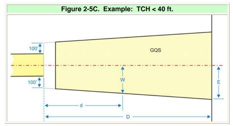
Calculate the GQS half-width "E" at the DA point measured along the runway centerline extended using the following formula:
