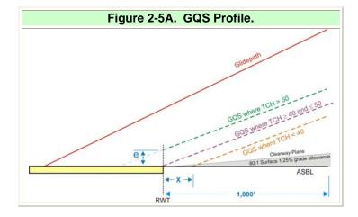
**2.12.1 b. Width**. The GQS lateral boundary is 100 ft from the runway edge at RWT. It expands uniformly to a width of "E" feet at DA (see figures 2-5B and 2-5C).
