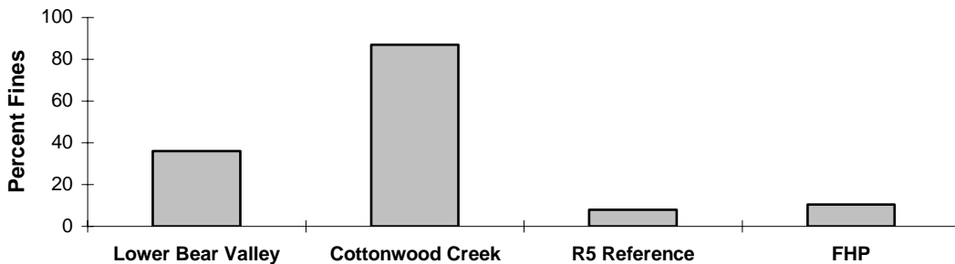
Figure 2 - SCI data comparison of Pool Tail Surface Fines for transport reaches within the Cottonwood Fire against R5 reference and FHP streams.
