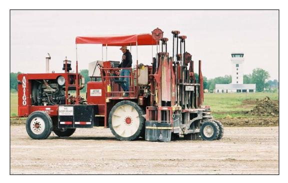
Figure 2. Multi-Head Breaker Machine
