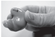
Clean canal portion of the hearing aid.
