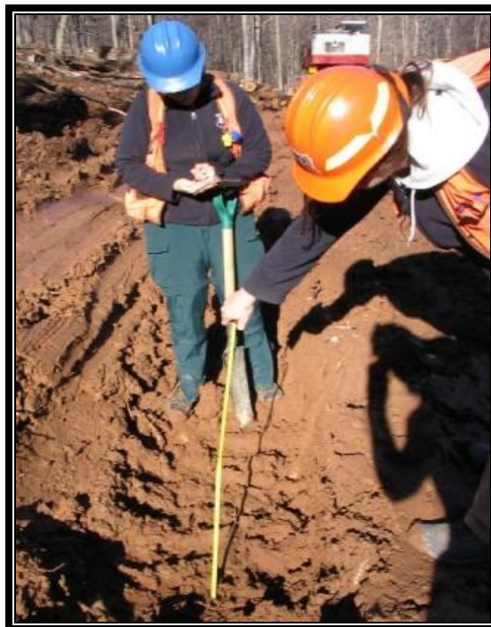
Figure SL-4. Monitoring Crew Measuring Depth of Rut in Pay Unit 2
