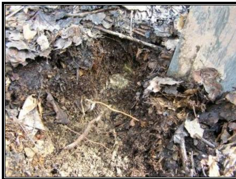
Figure SL-7. Soil profile (O horizon, A horizon, B horizon) in colluvium in ephemeral stream within burned unit 4/16/07
