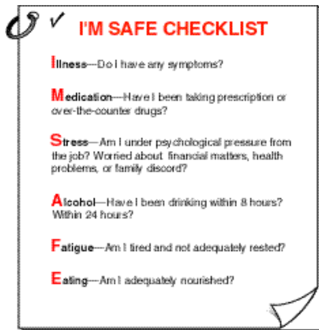
Figure 9-9. Prior to flight, pilots should assess their fitness, just as they evaluate the aircraft's airworthiness.
