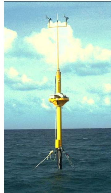
A typical Coral Reef Early Warning System (CREWS) station.
