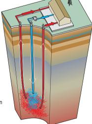
**Right:** Schematic diagram of an enhanced geothermal system
