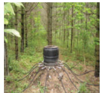
Right: The infrasound "spider" array, located at the Elgin Field Observatory, Ontario, Canada, detects low frequency acoustic waves generated by atmospheric explosions..
