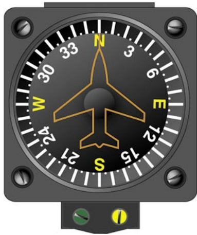
Figure 3-22. Vertical Card Magnetic Compass.
