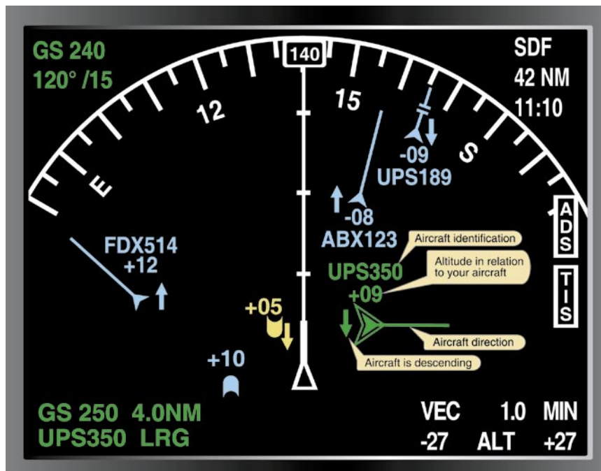
Figure 3-49. An aircraft equipped with ADS will receive identification, altitude in hundreds of feet (above or below using + or -), direction of the traffic, and aircraft descent or climb using an up or down arrow. The yellow target is an illustration of how a non-ADS equipped aircraft would appear on an ADS-equipped aircraft's display.
