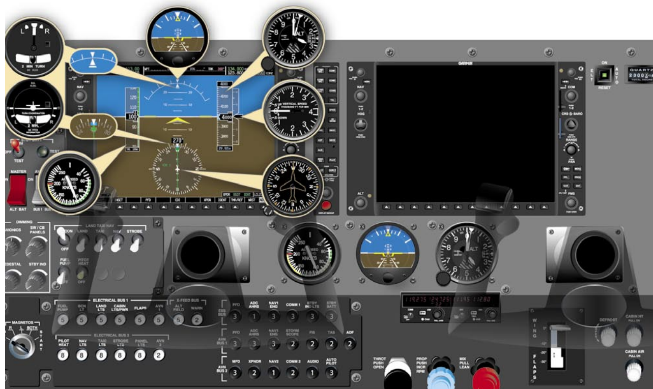
Figure 4-21. Primary Flight Display (PFD) and Analog Counterparts.
