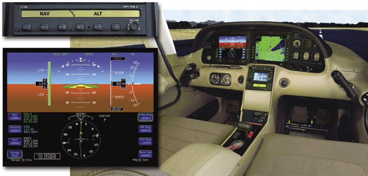
Figure 3-41. The S-TEC/Meggitt Corporation Integrated Autopilot Installed in the Cirrus.
