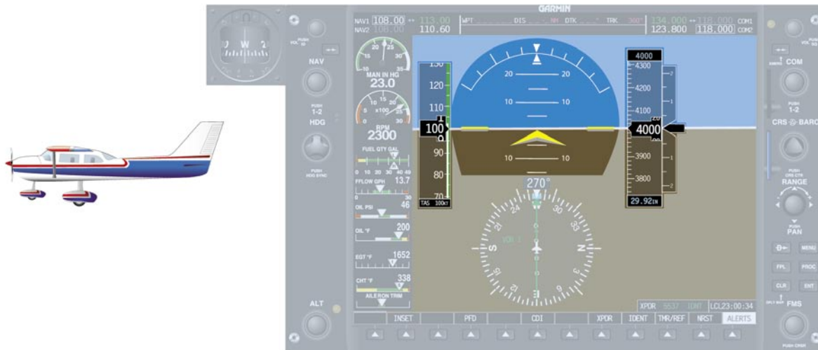
Figure 4-30. Pitch of the Aircraft.
