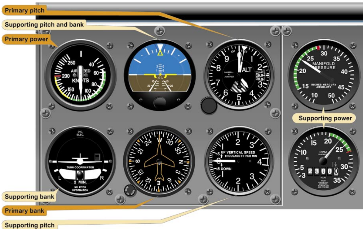
Figure 5-22. Straight-and-Level Flight (Normal Cruising Speed).
