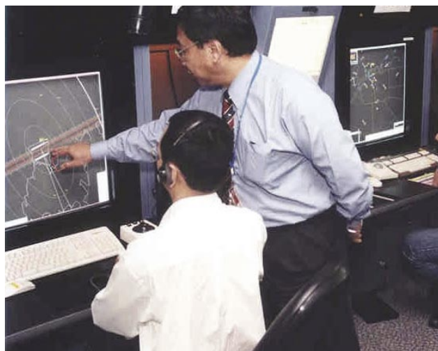
Figure 9-14. High Resolution ATC Displays Used in PRM.
