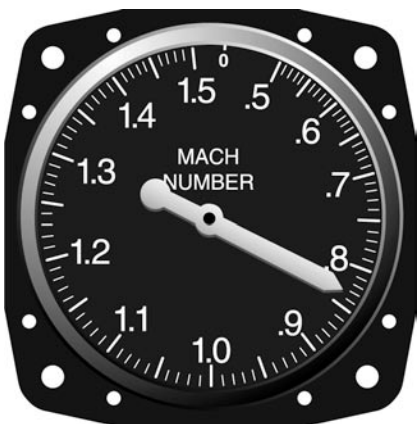
Figure 3-13. A Machmeter shows the ratio of the speed of sound to the TAS the aircraft is flying.
