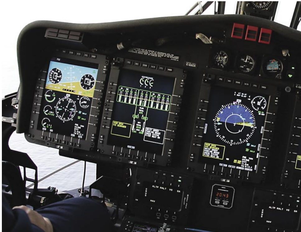
Figure 6-20. MFD Display of Aircraft Systems.
