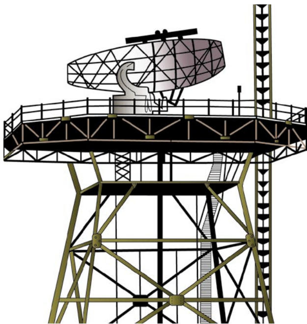
Figure 9-7. Combined Radar and Beacon Antenna.
