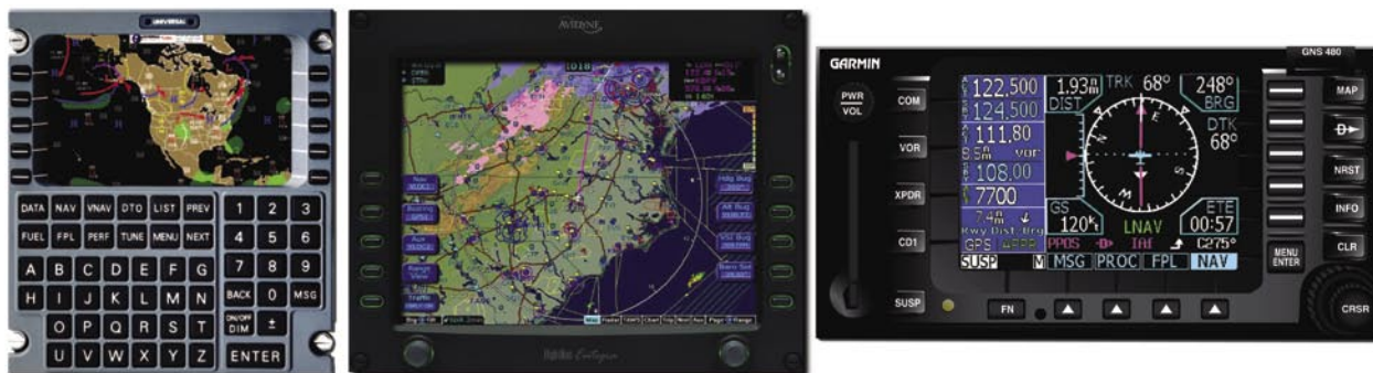
Figure 7-43. Typical Display and Control Unit(s) in General Aviation. The Universal UNS-1 (left) controls and integrates all other systems. The Avidyne (center) and Garmin systems (right) illustrate and are typical of completely integrated systems. Although the Universal CDU is not typically found on smaller general aviation aircraft, the difference in capabilities of the CDUs and stand-alone systems is diminishing each year.
