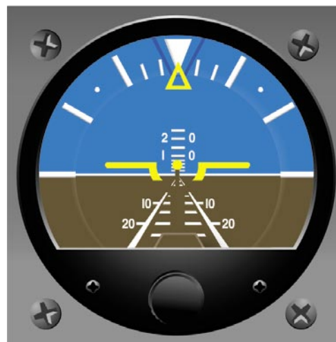
Figure 5-5. Pitch Correction for Level Flight, One Bar Width.
