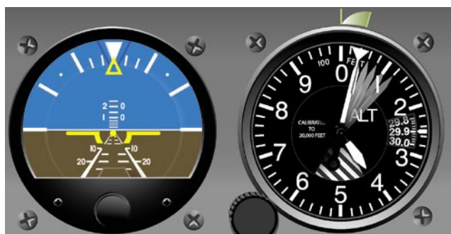
Figure 5-8. Pitch Correction Following Altitude Increase—Lower Nose to Correct Altitude Error.
