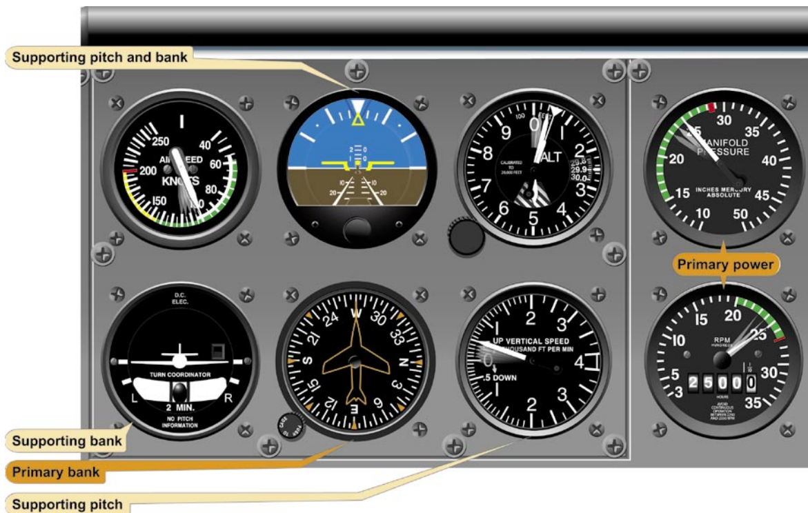
Figure 5-25. Climb Entry for Constant Airspeed Climb.
