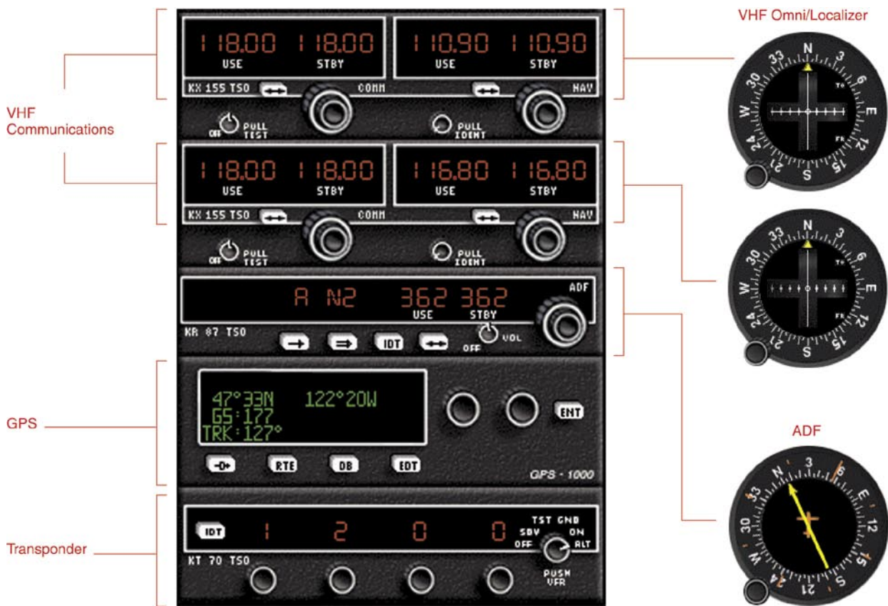
Figure 9-1. Typical NAV/COM Installation.
