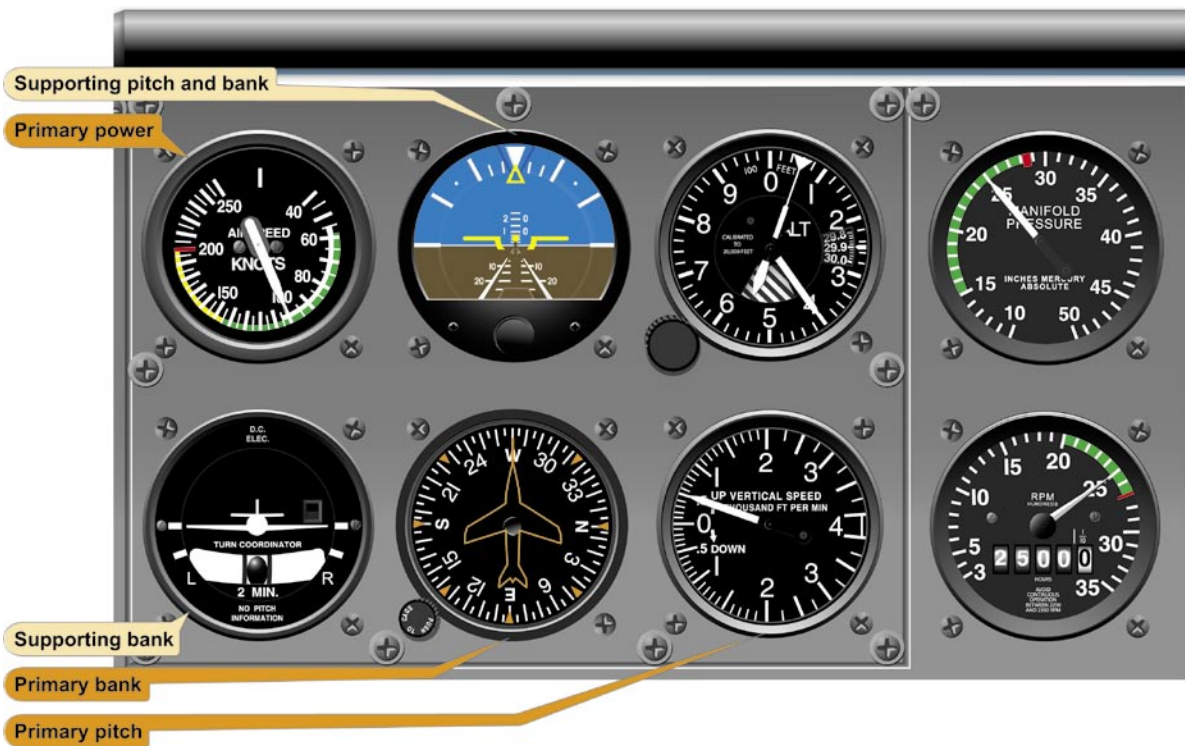
Figure 5-27. Stabilized Climb at Constant Rate.
