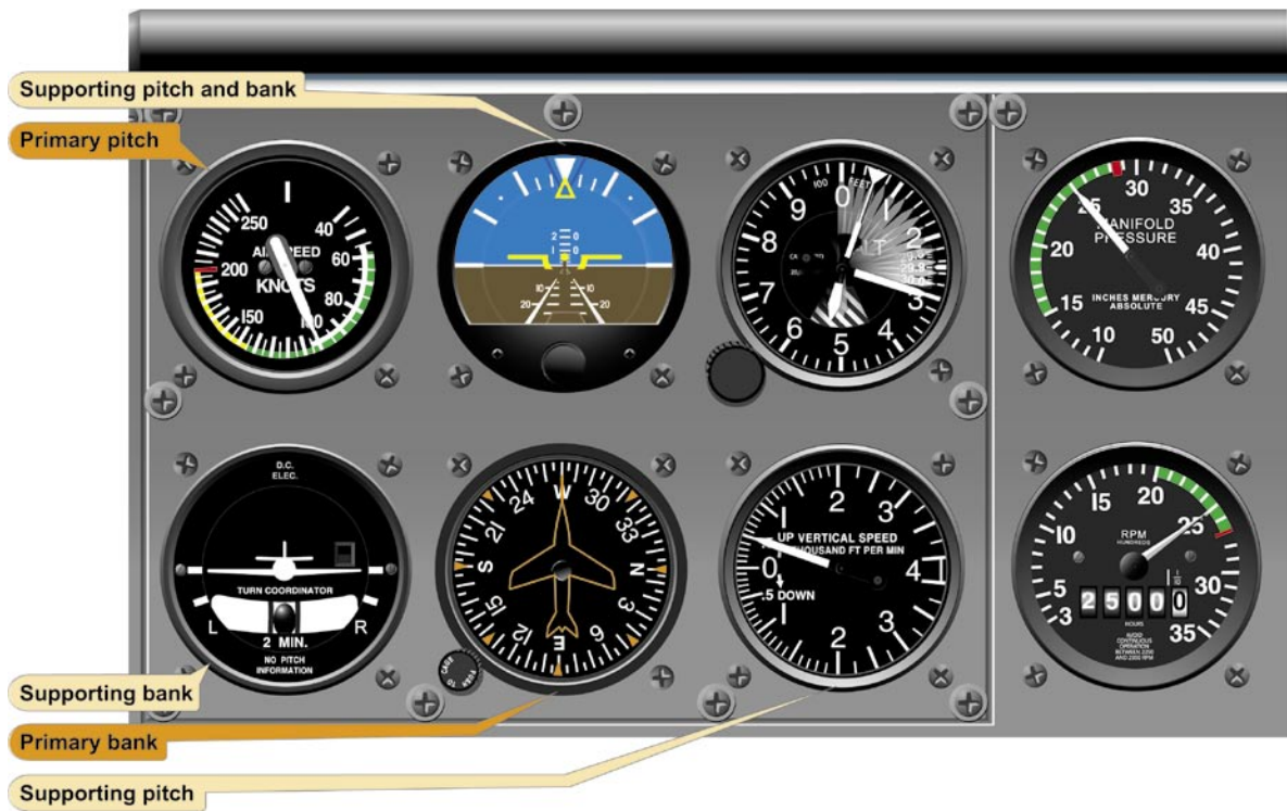
Figure 5-26. Stabilized Climb at Constant Airspeed.
