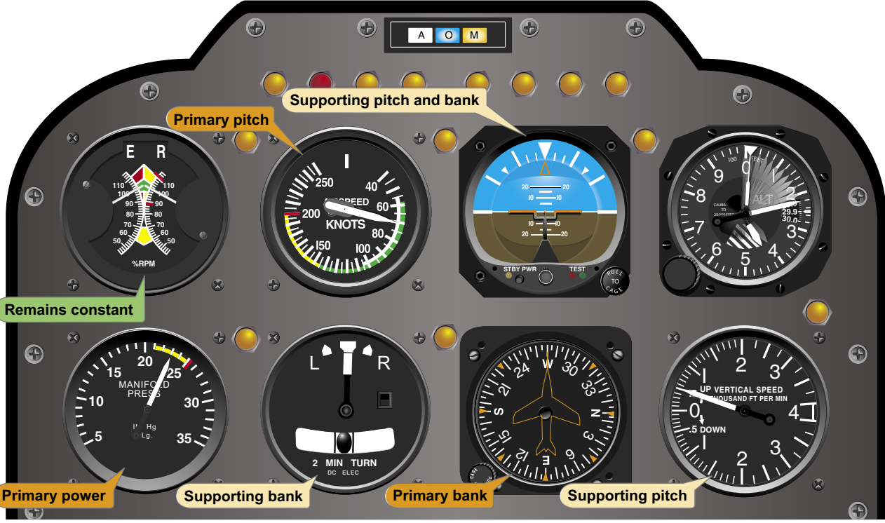
Figure 6-12. Flight instrument indications in a stabilized constant-airspeed climb.
