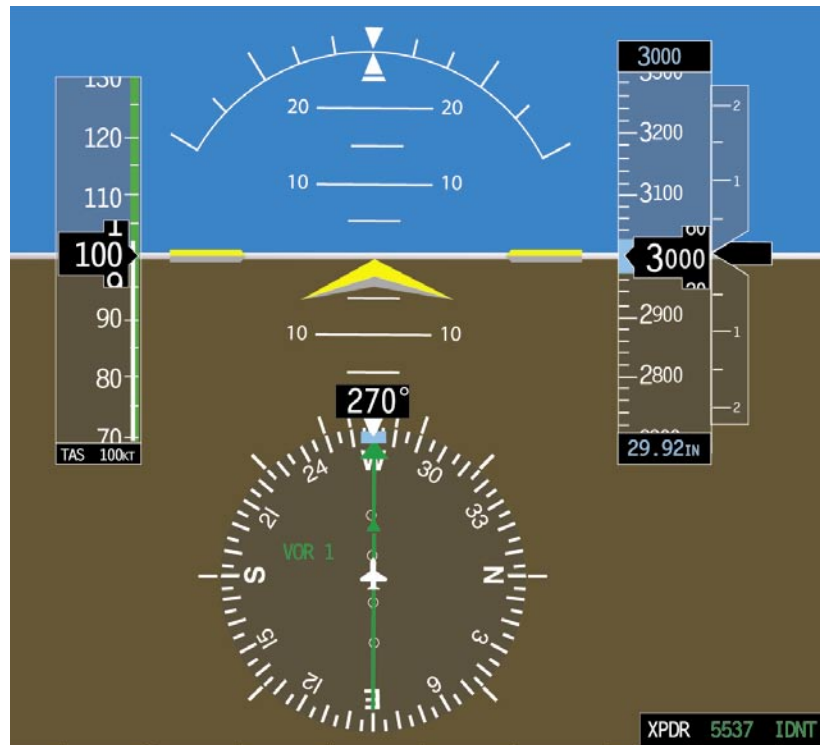
Figure 6-17. PFD Indications During Straight-and-Level Flight.
