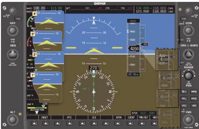
Figure 5-50. Pitch Indications for Various Attitudes (1° through 5°).
