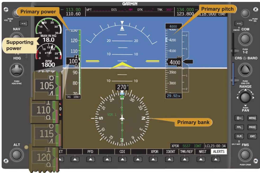
Figure 5-59. Straight-and-Level Flight (Reduced Airspeed Stabilized).
