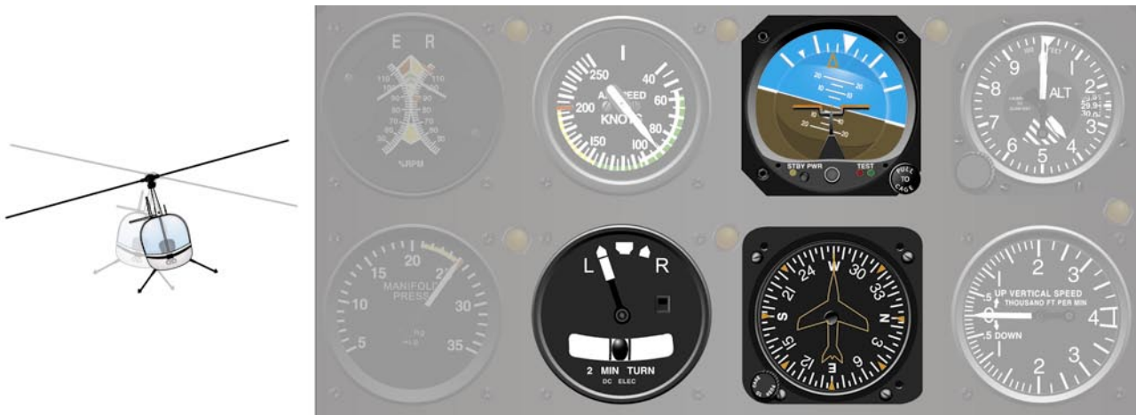
Figure 6-4. The flight instruments used for bank control are the attitude, heading, and turn indicators.
