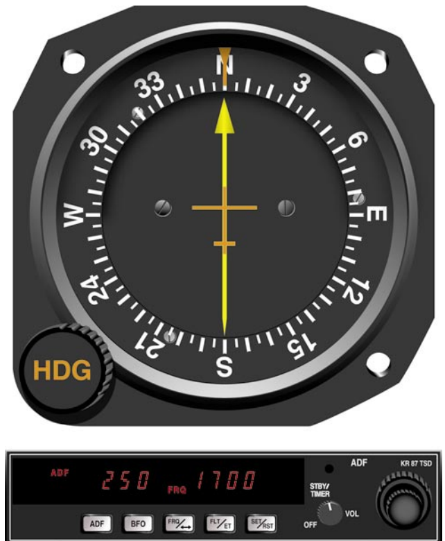
Figure 7-2. ADF Indicator Instrument and Receiver.
