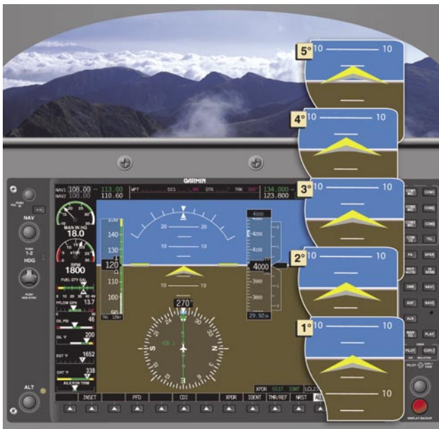
Figure 5-49. Various Pitch Attitudes (Right), Aircraft Shown in Level Flight.
