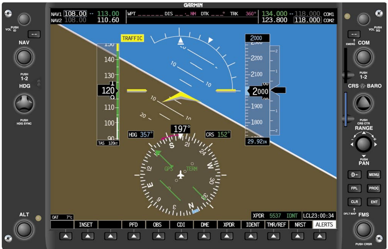
Figure 4-39. Horizontal Situation Indicator (HSI) Trend Indicator Elongates Proportionally With the Rate of Turn.
