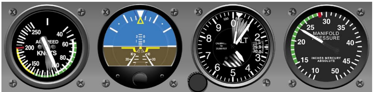
Figure 5-20. Airspeed Low and Altitude High—Lower Pitch.
