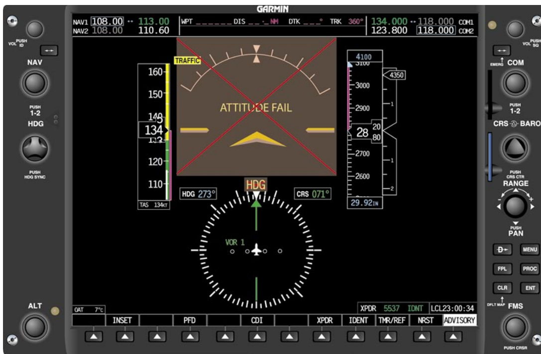
Figure 5-73. AHRS Unit Failed.
