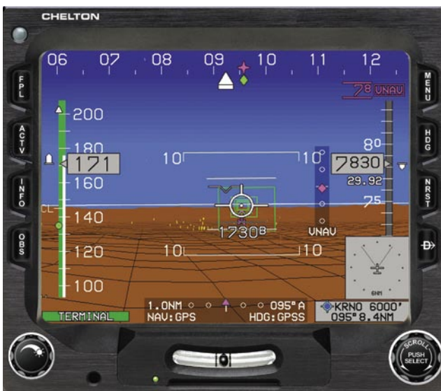
Figure 3-46. The benefits of realistic visualization imagery, as illustrated by Synthetic Vision manufactured by Chelton Flight Systems. The system provides the pilot a realistic, real-time, three-dimensional depiction of the aircraft and its relation to terrain around it.
