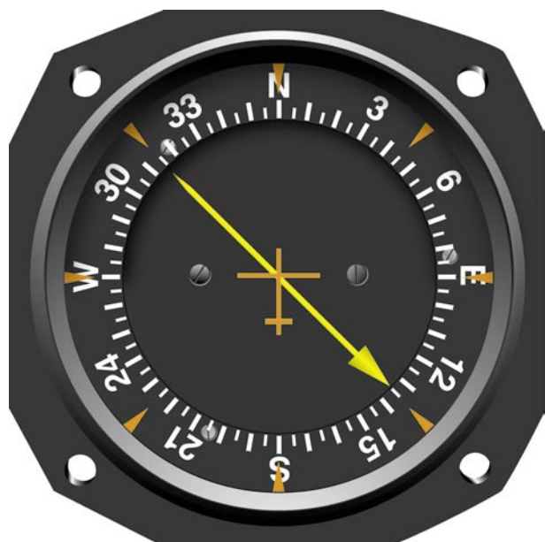
Figure 7-3. Relative bearing (RB) on a fixed-card indicator. Note that the card always indicates 360°, or north. In this case, the relative bearing to the station is 135° to the right. If the aircraft were on a magnetic heading of 360°, then the magnetic bearing (MB) would also be 135°.
