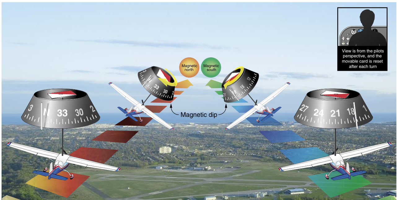
Figure 3-20. Northerly Turning Error.
