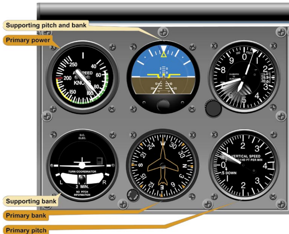
Figure 5-28. Airspeed Low and Vertical Speed High—Reduce Pitch.
