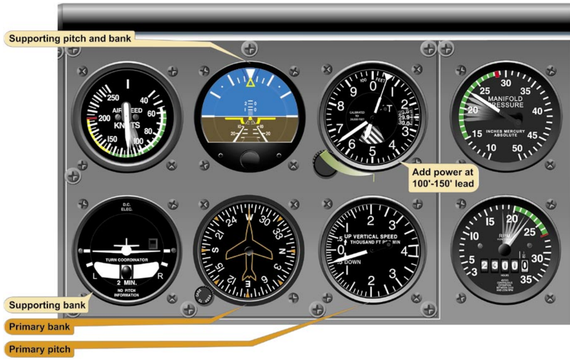
Figure 5-31. Level Off Airspeed Higher Than Descent Airspeed.
