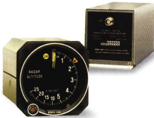
Figure 3-51. Components of a Radar Altimeter.
