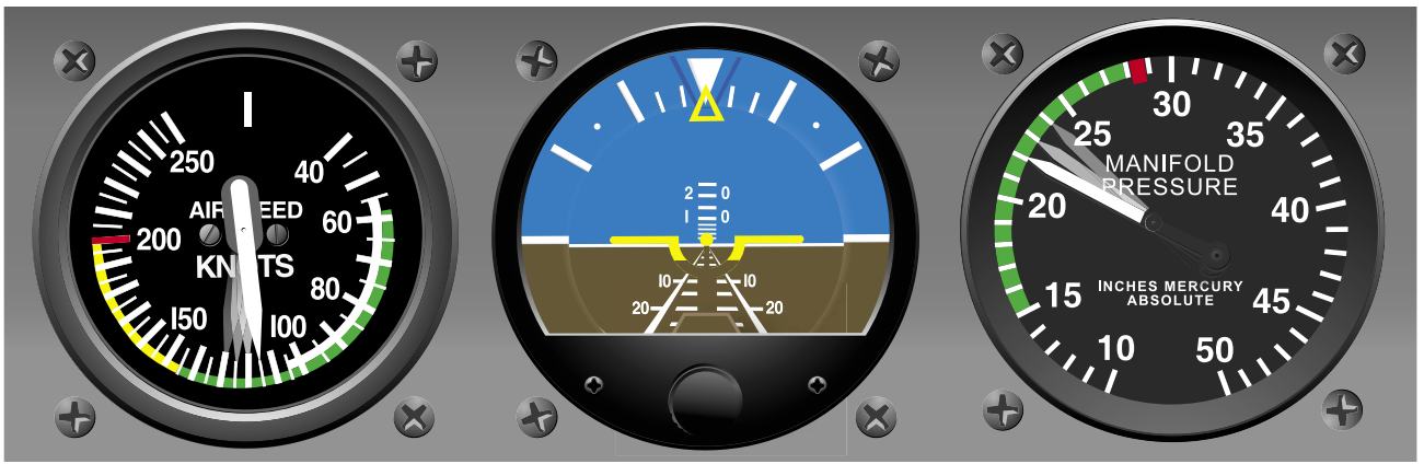
Figure 4-14. Pitch Control and Power Adjustment Required To Bring Aircraft to Level Flight.
