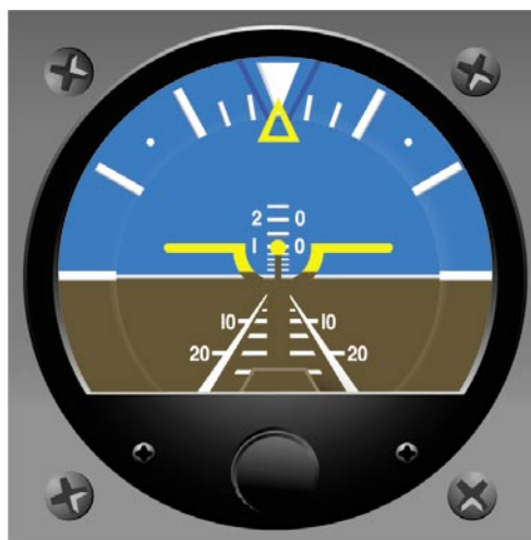
Figure 5-6. Pitch Correction for Level Flight, One-and-One-Half Bar Width.
