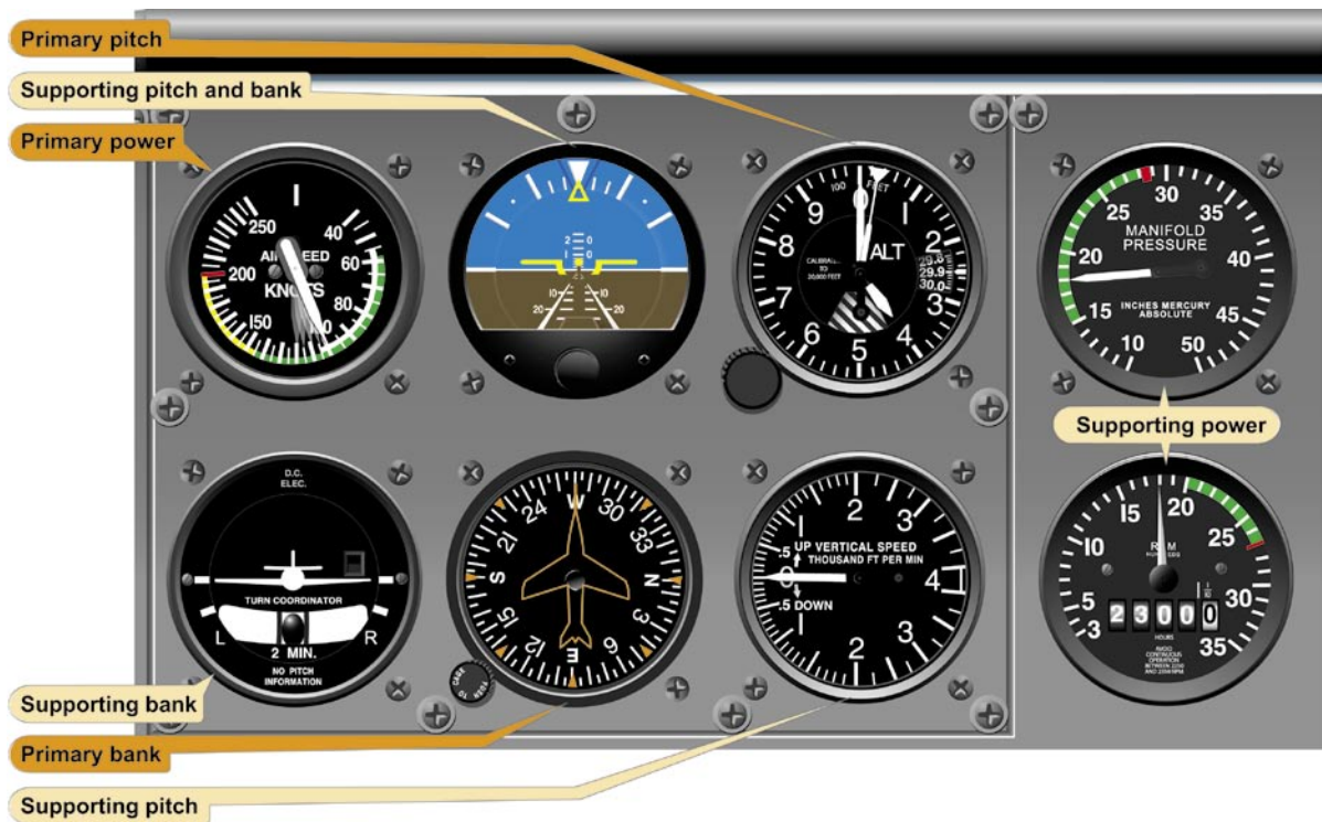
Figure 5-24. Straight-and-Level Flight (Reduced Airspeed Stabilized).
