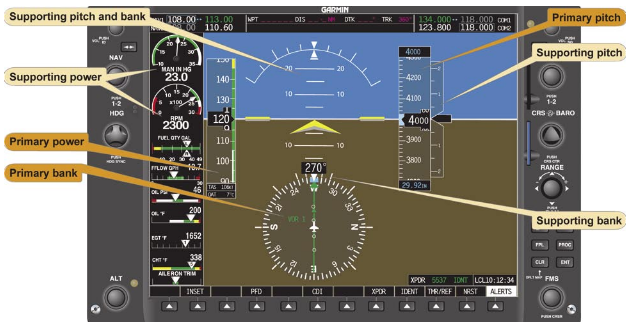
Figure 5-57. Straight-and-Level Flight (Normal Cruising Speed).
