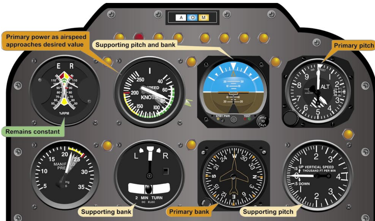
Figure 6-10. Flight instrument indications in straight-and-level flight with airspeed decreasing.
