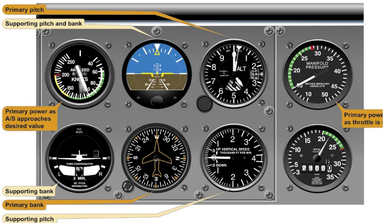
Figure 5-23. Straight-and-Level Flight (Airspeed Decreasing).
