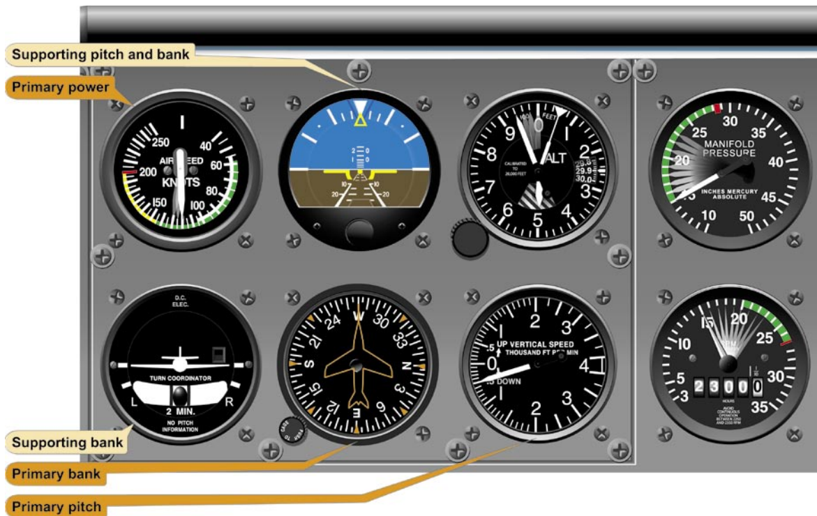
Figure 5-30. Constant Airspeed Descent, Airspeed High—Reduce Power.
