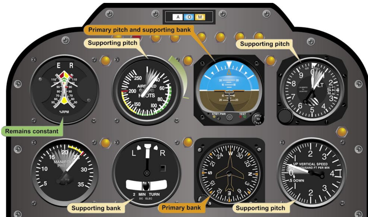
Figure 6-16. Flight Instrument Indications During an Instrument Takeoff.
