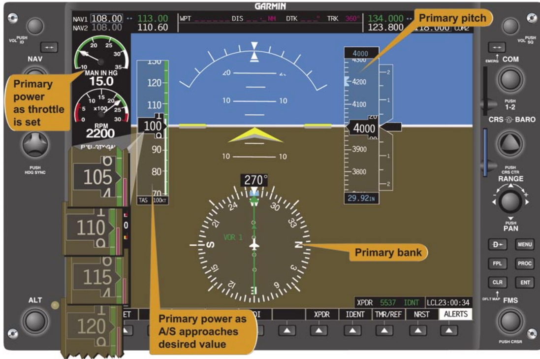
Figure 5-58. Straight-and-Level Flight (Airspeed Decreasing).
