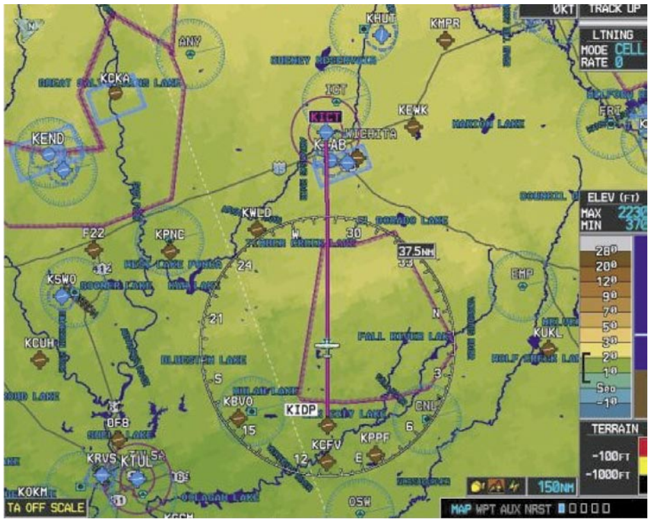
Figure 6-19. MFD Display of a Moving Map.
