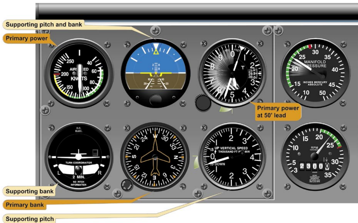
Figure 5-32. Level Off at Descent Airspeed.
