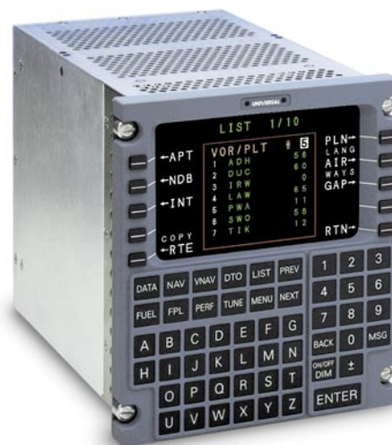
Figure 3-44. A Control Display Unit (CDU) Used to Control the Flight Management System.
