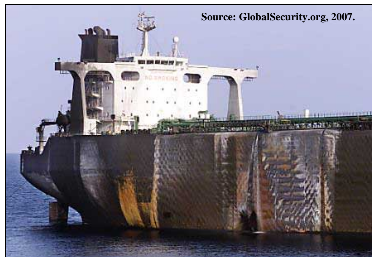
Figure 65. Damage to the Limburg Following Terrorist Attack.
