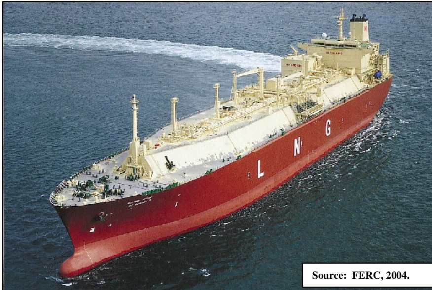
Figure 59. LNG Tanker with Prismatic Tanks.
