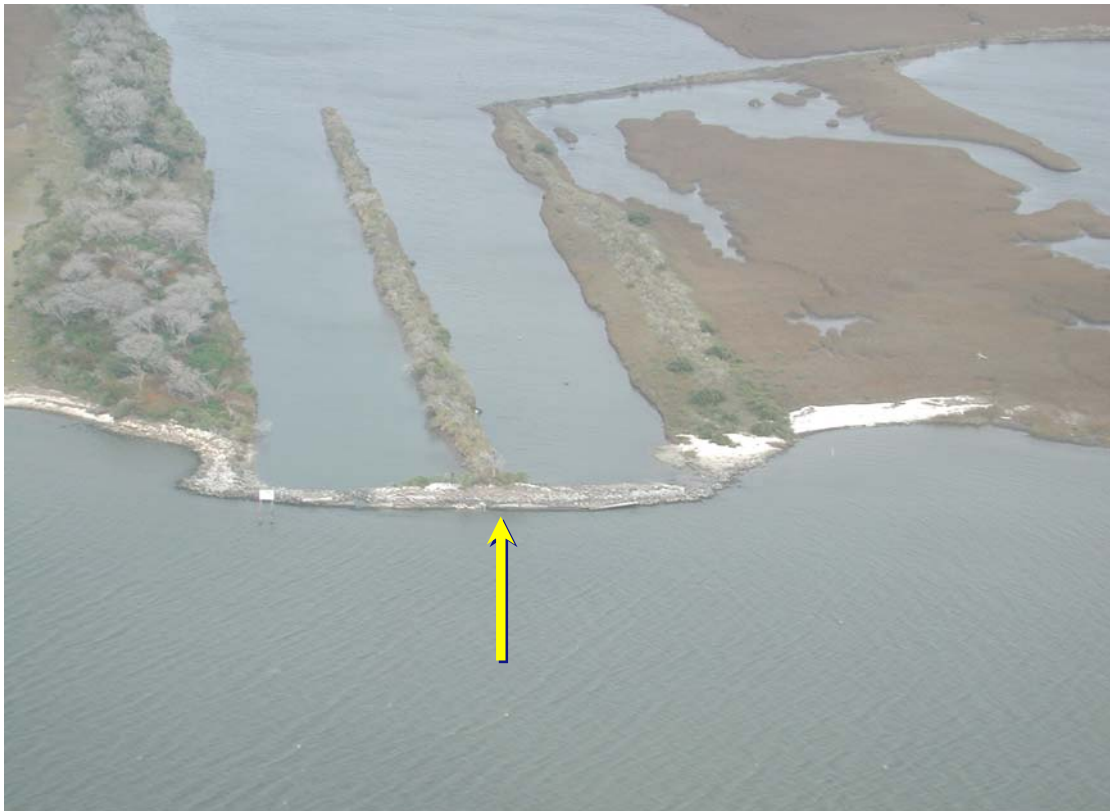
Figure 11-c. Aerial photograph taken on 7 February 2004 of riprap used to plug the pipeline canals. Note the gravel beach to the east (right) of the structure, and that it was not possible to differentiate between the riprap and gravel using the IKONOS imagery classification.
