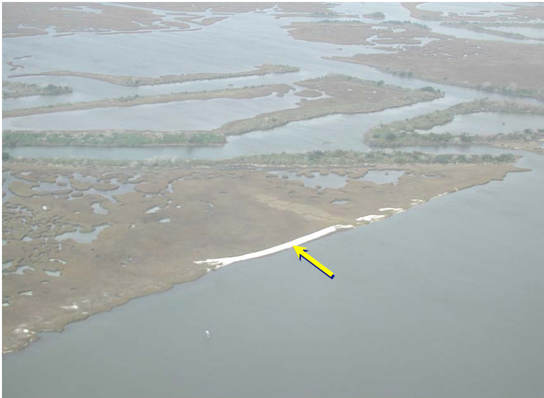
Figure 10-c. Aerial photograph taken on 6 February 2004 of a gravel (shell) beach along Bayou Lafourche. The bright white oyster shells occur as washover berm on the marsh surface created by large boat wakes along waterways with heavy traffic by large vessels.
