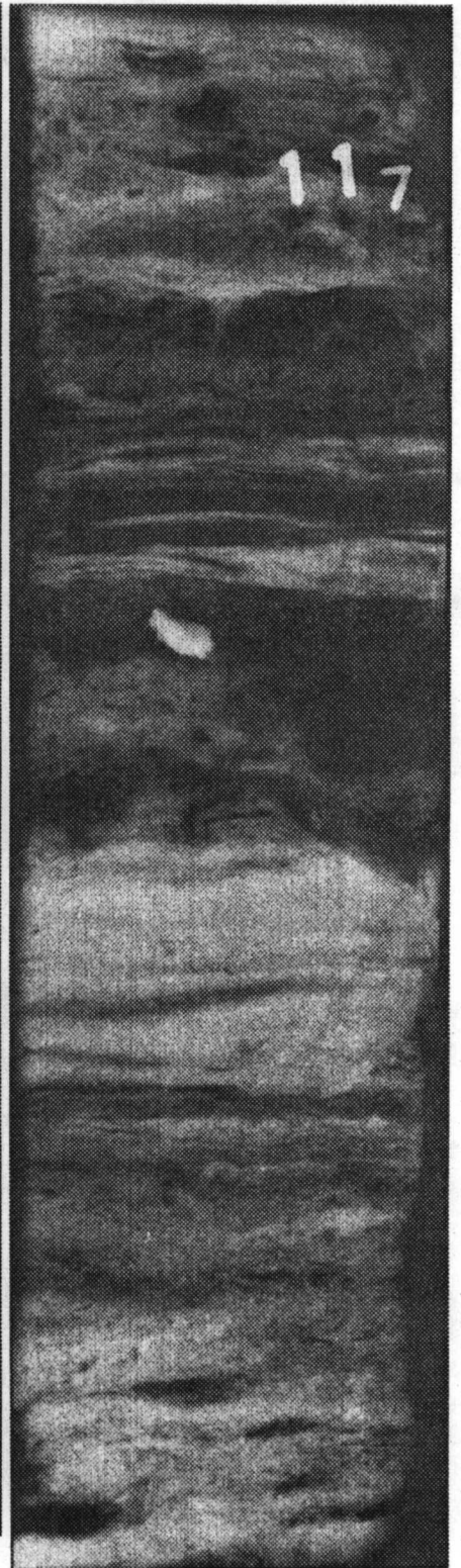
Figure 7.44. Beach ridge and bay sediments characteristic of the infilling of the Muskrat Line pipeline canal shown on vibracore 4 (east end) at 1.2 to 1.5 m (A) and vibracore 1 (west end) at 1.3 to 0.6 m (B).
