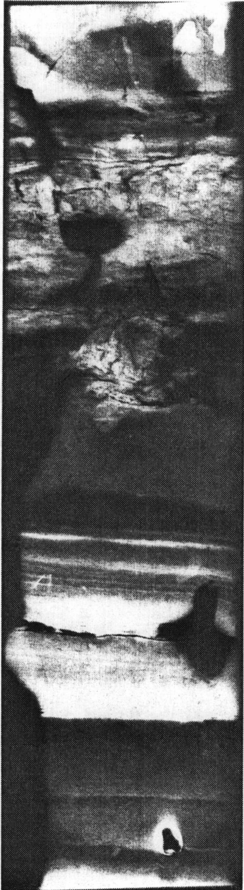
Figure 7.54. PR3 radiograph of channel sediments at 2.4 to 2.7 m at the control site.
