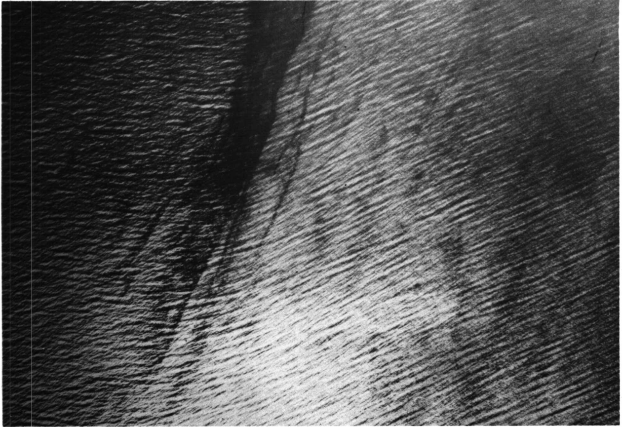
Figure 7.26A. Wave refraction data in a U-2 aerial photo taken near the CA coast. (Water depth is 90 m and dominant wavelength is about 100 m. The front was about 1 km wide.)
