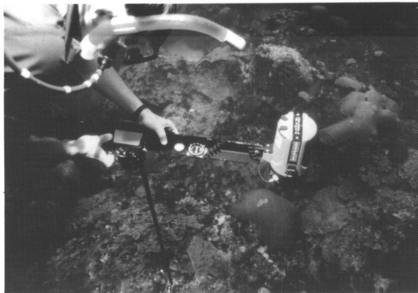
Figure 2.3. Compass and bubble level mounted on the top of the T-frame used to photograph each 8\text{m}^2 repetitive station. (These are used to adjust attitude of unit at each station prior to photography).
