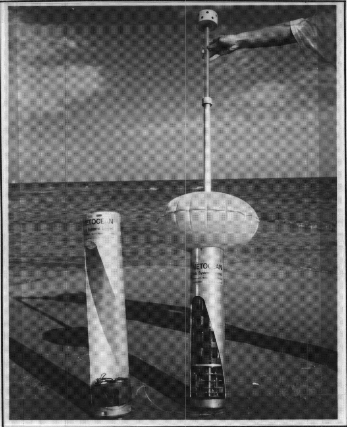
Figure 13.2. A fully deployed buoy (cut open to show insides). (The surface unit is on the right, and the launch container on the left. The surface unit houses the air-pressure port and air temperature sensor in a white knob at the top [above the antenna]. The sea-surface temperature sensor is at the bottom of the surface unit. The subsurface temperature cable is still on the spool at the bottom of the launch container. All electronics [data sampling, averaging, transmitter] are on five circular boards at the bottom of the surface unit. Above these boards is the power stack of C-cell batteries.)
