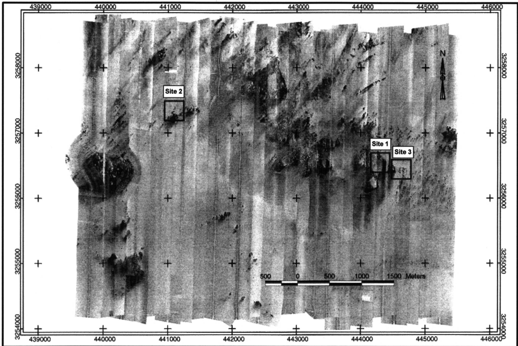
Fig. 4.10. TAMU 2 side-scan sonar mosaic of Megasite 1, showing Monitoring Sites 1-3 (small boxes). Vertical stripes are individual trackline side-scan sonar records pieced together to make the mosaic. Dark areas are high acoustic return (backscatter), whereas light areas are low backscatter. UTM plot with axes labeled in meters.
