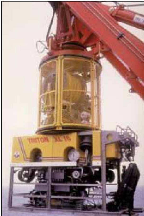
Photo 3-1 - Triton remotely operated vehicle (ROV) with launch and recovery system (LARS) and tether management system (TMS) used during the Screening Cruise.
