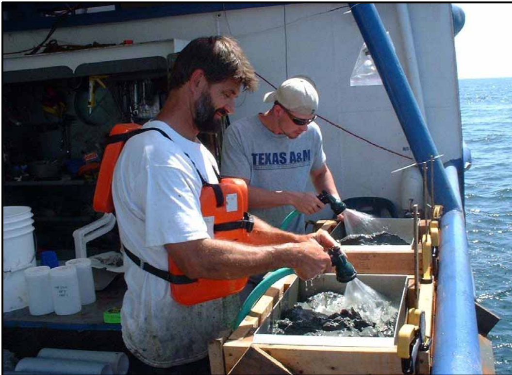
Photo 3-7 - Washing macrofaunal samples through 0.5-mm wire mesh sieves.
