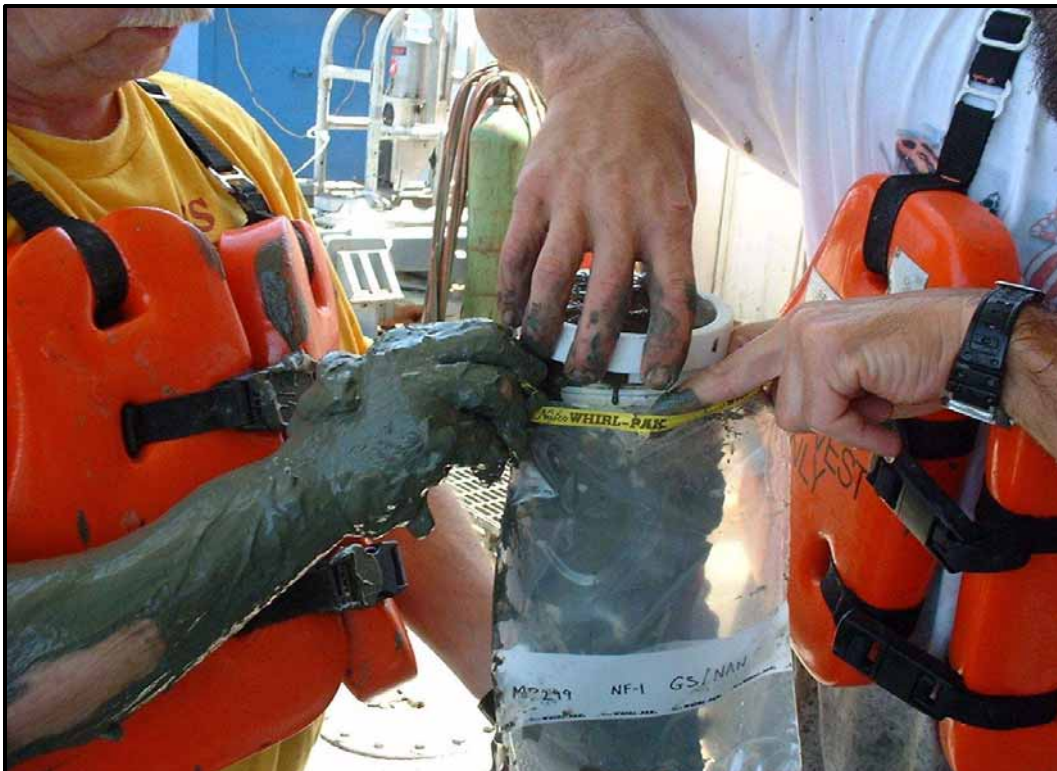
Photo 3-6 - Collection of 2-cm subsurface samples from a Teflon® core tube.
