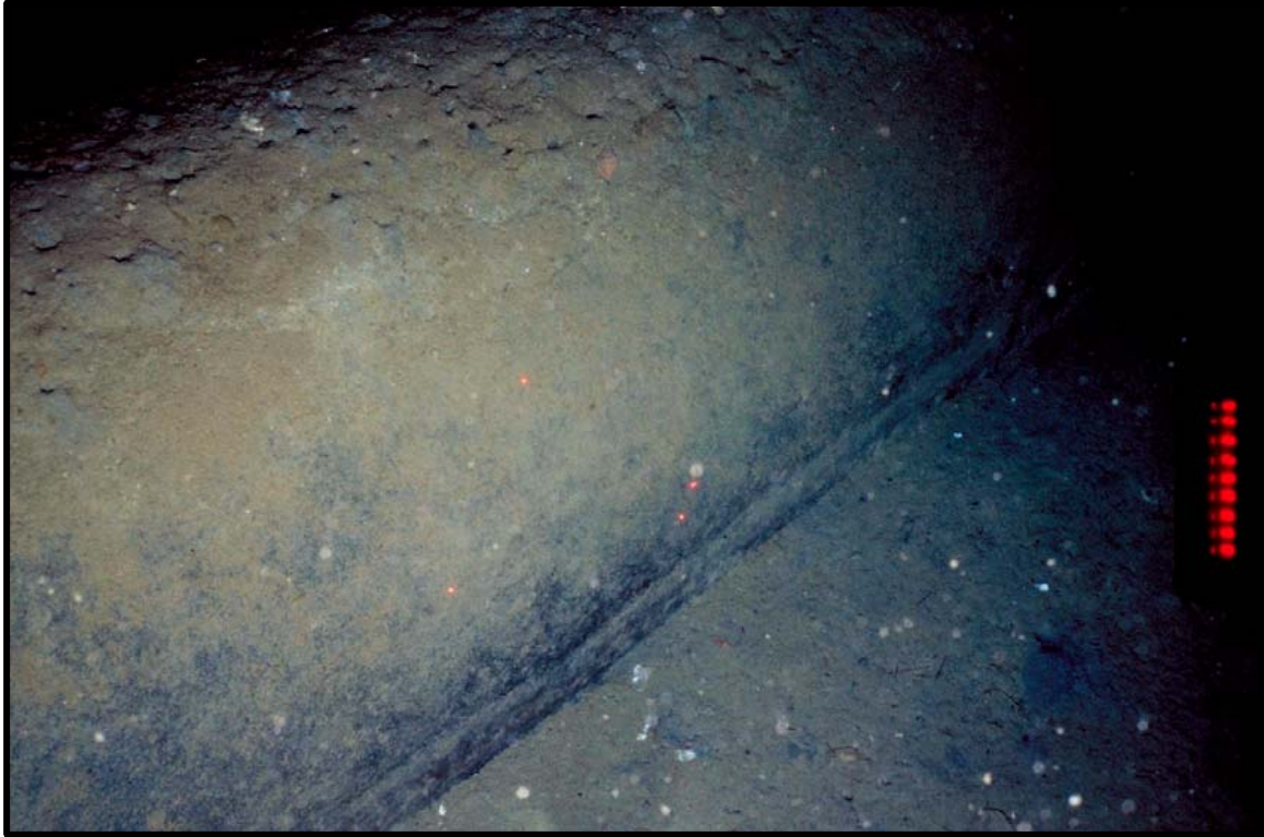
Photo 2-25 - Accumulation of suspected discharge material along the northeast Viosca Knoll 780 platform. Depths of the observed accumulation ranged from approximately a few inches to a slight dusting.
