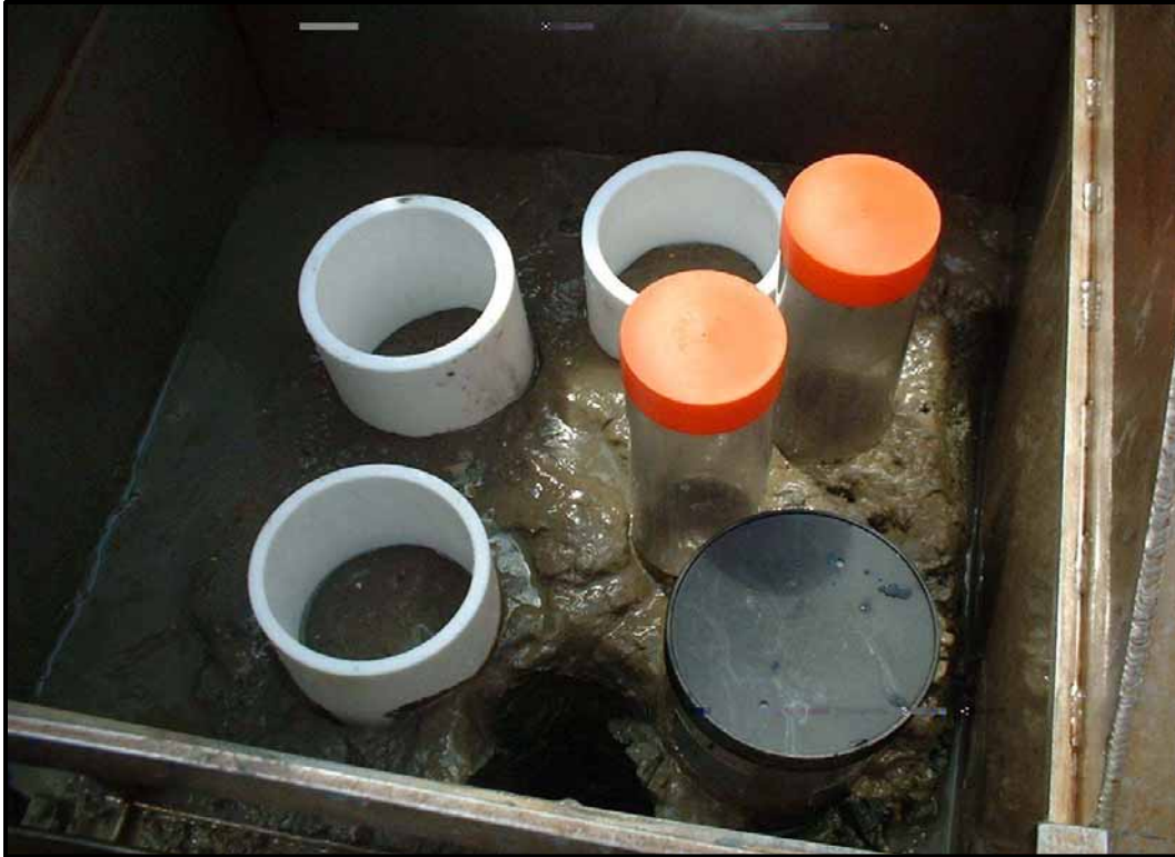
Photo 3-5 - Placement of Teflon® and acrylic core tubes within a box core sample.
