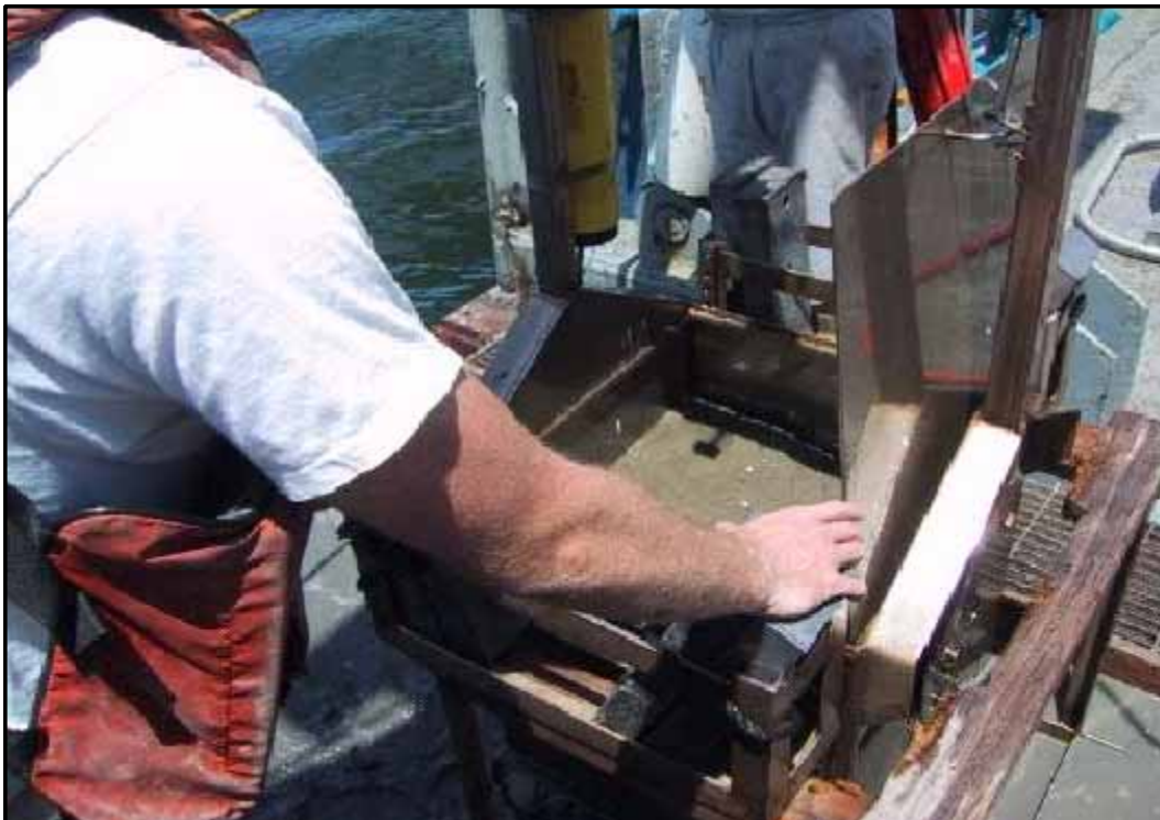
Photo 3-4 - Visual inspection of the surface layer and integrity of a box core sample.
