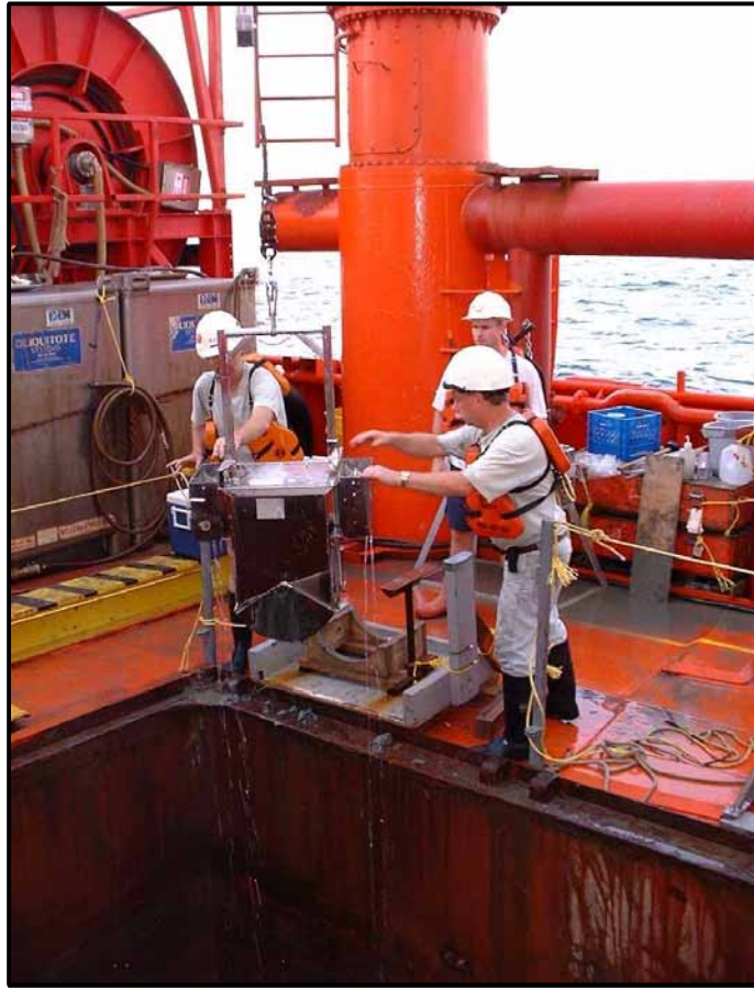
Photo 3-3 - Retrieval of the box core during the Screening Cruise.
