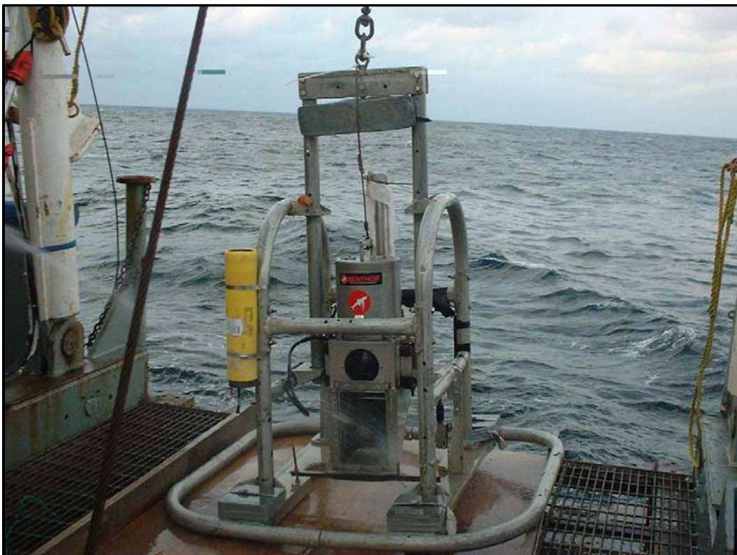
Photo 3-8 - Sediment profile imaging (SPI) camera and frame. Sonardyne® beacon (yellow) shown mounted on SPI frame leg.
