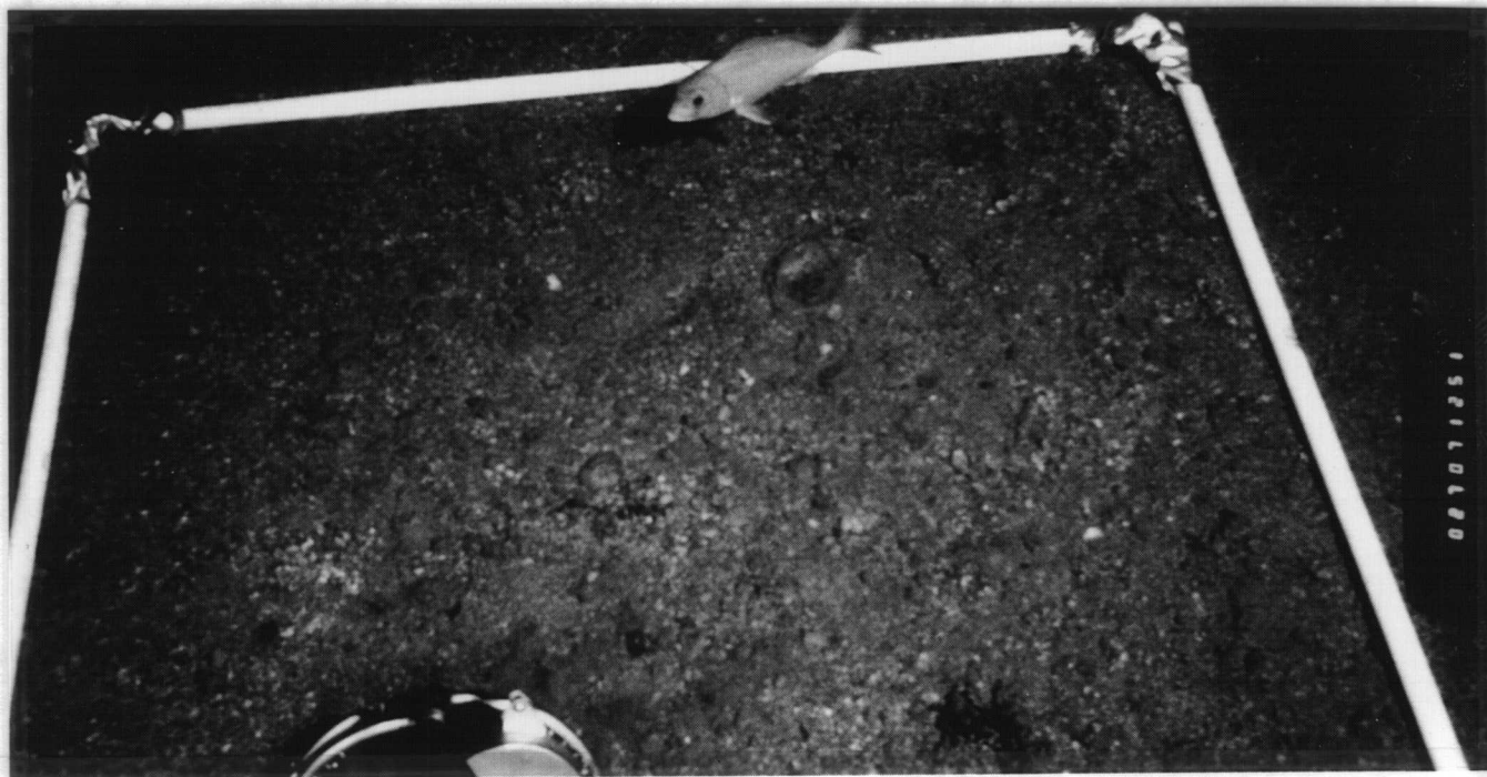
Figure 5. Photo at Pensacola No. 1 taken with external camera showing 1-m 2 PVC frame with sampling scoop in lower left. Sediment is a mixture of cuttings and natural sediment. Note clump of fleshy algae near right bottom and large pelecypod shell beneath fish.
