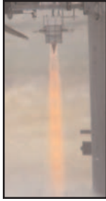
Aerospike engine static fire test
