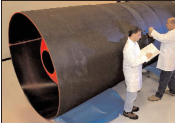
Subscale Composite Cryogenic Tank
