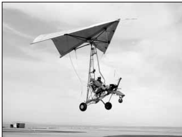
Figure 1-4. NASA testing the Rogallo wing, which led to the modern hang glider and WSC aircraft.
