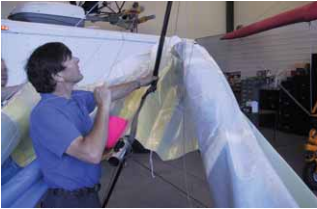
Figure 5-19. Raising the kingpost and spreading the wings as needed to keep the kingpost upright.
