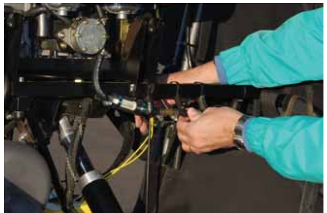
Figure 5-54. Checking the security and condition of the fuel lines and fuel filter condition.
