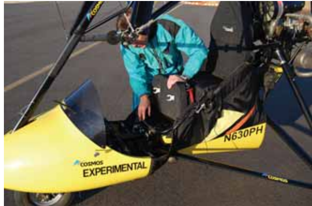
Figure 5-49. Inspecting the front keel and seat attachments to the keel.
