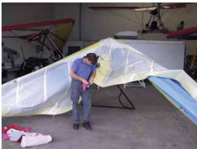
Figure 5-34. Padding the keel and kingpost with the right hand sail over the top of the leading edge.
