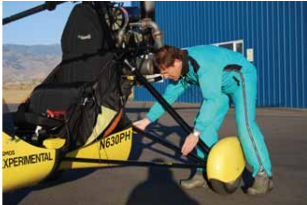
Figure 5-51. Checking the rear landing gear struts.
