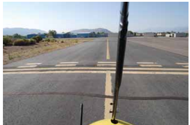
Figure 5-66. Taxi on the airport yellow taxi line, but stop at the “hold short line” to get clearance before taxiing across or onto an active airport runway.
