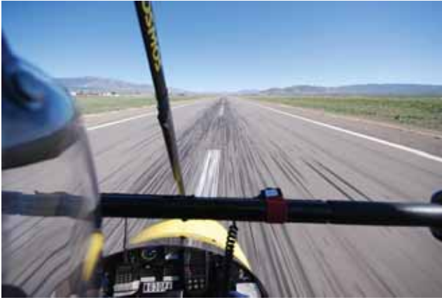
Figure 11-13. Continuing the roundout as speed bleeds off and the WSC back wheels are inches above the runway.
