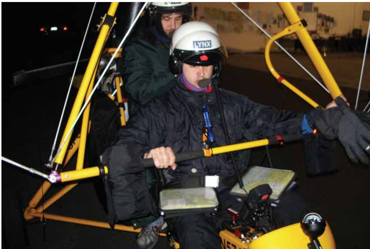
Figure 12-5. WSC aircraft equipped for night cross-country flight with flashlight and aeronautical charts on kneeboards.
