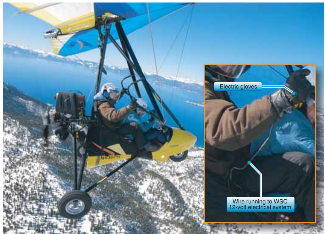
Figure 1-21. Motorcycle gloves and socks hooked to the 12-volt WSC electrical system keep the pilot and passenger warm.
