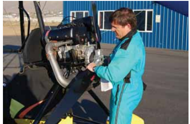
Figure 5-53. Checking the security of the engine to the airframe.
