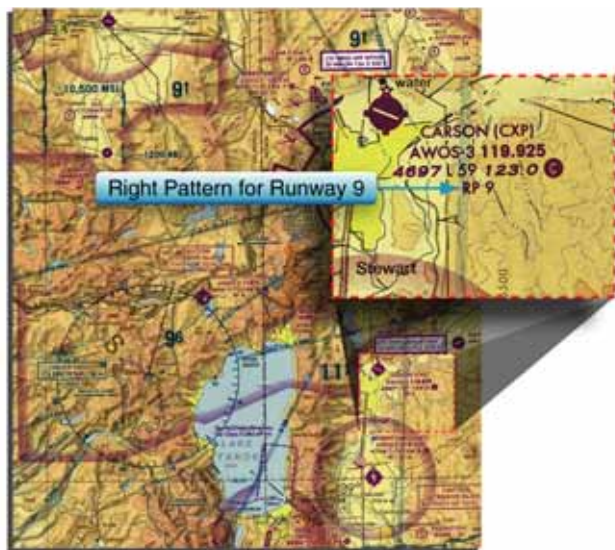
Figure 10-6. Example of traffic pattern indicator on sectional showing right hand pattern for runway 9. See Figure 10-5 for segmented circle for this airport.
