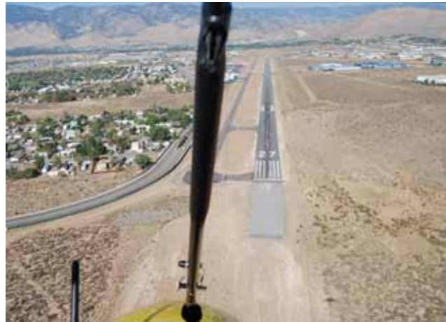
Figure 11-28. Pilot view of runway where a steep approach would be required.
