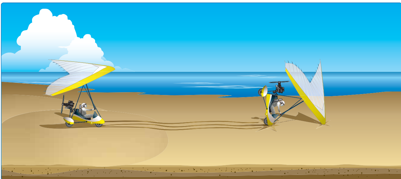
Figure 7-11. Soft field takeoff limitation for WSC aircraft: front wheel digs in and WSC aircraft rolls forward.
