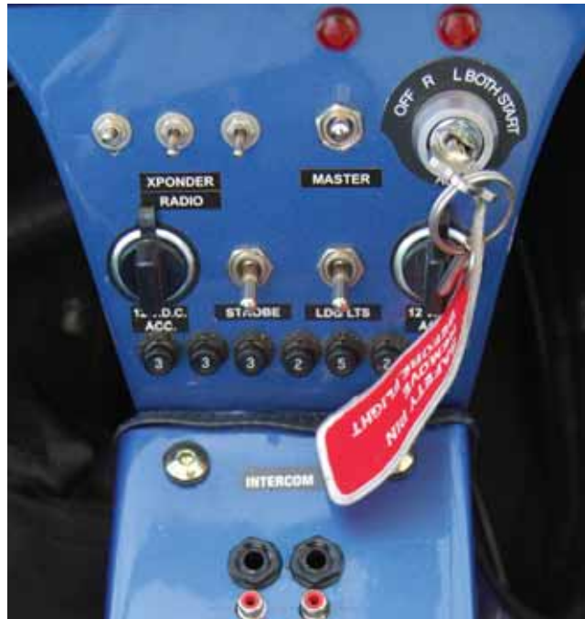
Figure 4-16. Keyed ignition system with integral starter.
