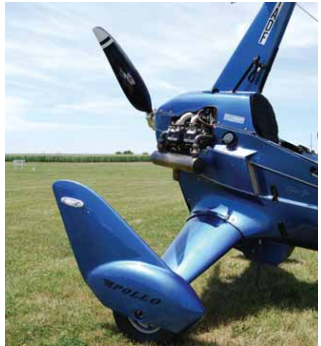
Figure 12-3. Modern LED position lights on carriage wheel pants simplify the installation with no wires running from the carriage to the wing tips.
