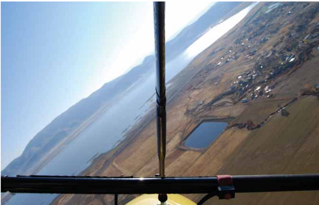
Figure 6-5. Pilot's view of 45° bank angle can be measured with the front tube or the control bar's angle with the horizon.
