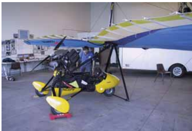
Figure 5-30. Wing in position and carriage chocked to lift the wing.
