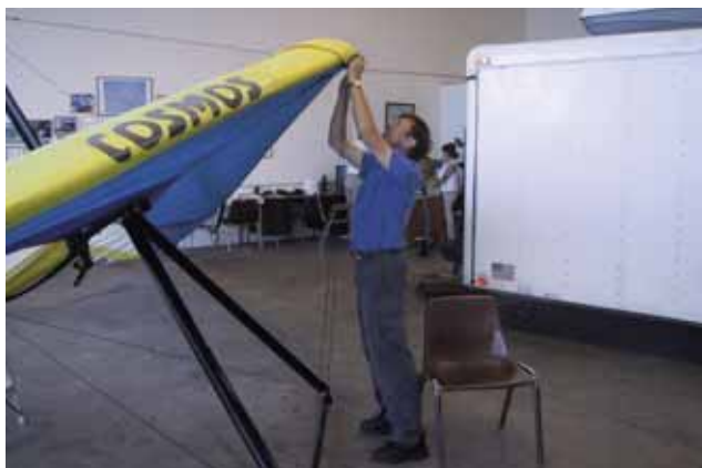
Figure 5-26. Attaching the front flying wires to the nose attachment.
