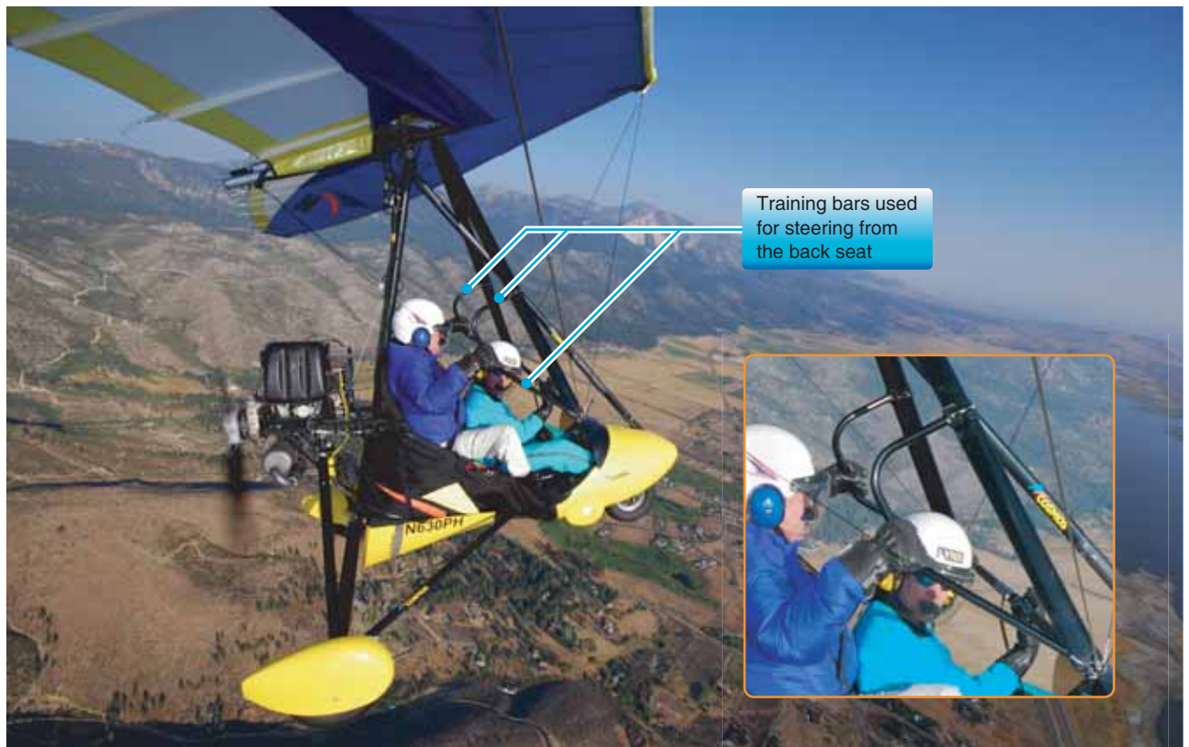
Figure 3-7. Passenger using training bars which are also used by the instructor during training.
