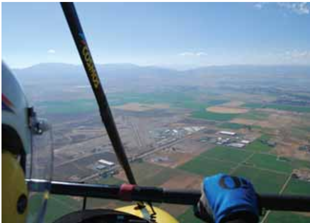
Figure 10-8. Approaching a busy airport with multiple runways and listening to the Common Traffic Advisory Frequency (CTAF) for the pattern being used because of the wind conditions.
