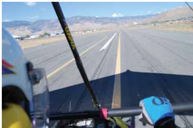
Figure 11-15. WSC aircraft follows the taxi line to exit the runway while slowing the aircraft and maintaining control of the wing.
