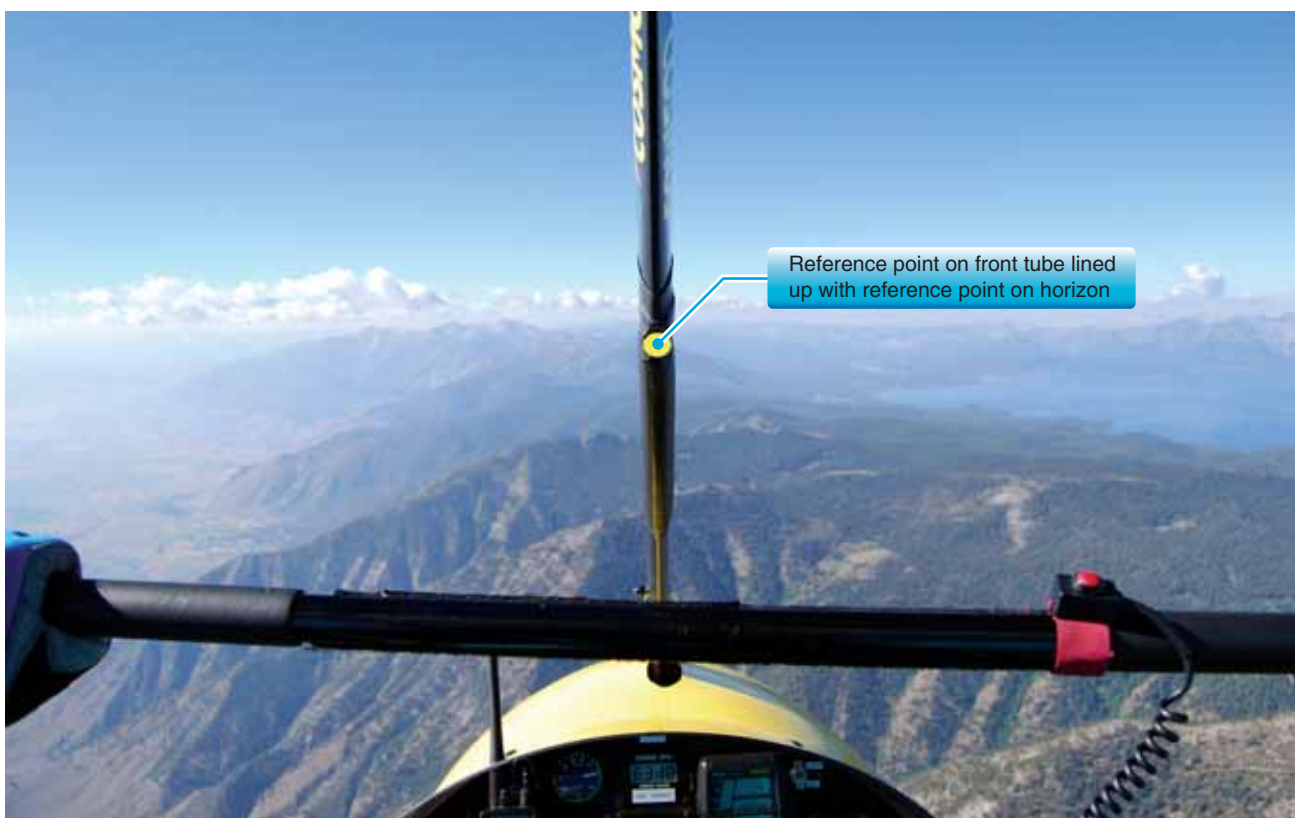
Figure 6-7. Pilot's view of a reference point on the front tube chosen for level flight and lined up with the reference point on the horizon for straight-and-level flight.
