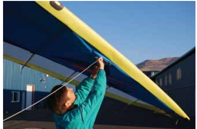
Figure 5-44. Inspecting the flying wire attachment to the leading edge and crossbar along with all the hardware at this junction.
