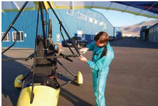
Figure 5-43. Inspecting the control frame brackets and flying wire attachments.
