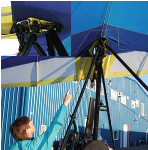
Figure 5-48. Inspecting the wing attachment to the carriage.
