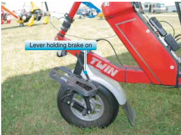
Figure 3-32. Mechanical parking brake system.
