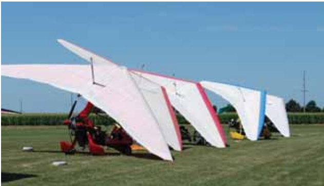
Figure 5-72. Group of WSC aircraft tied down with wing tips lowered into prevailing wind.
