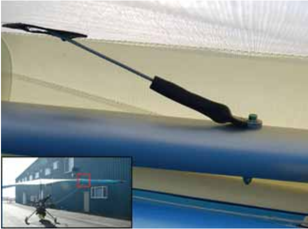
Figure 3-15. View inside wing showing top wire coming through sail that is reinforced, being attached to the crossbar by a tang, an aircraft bolt, washers, and lock nut.
