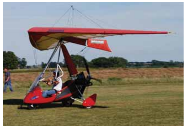
Figure 2-33. Keel pockets and horizontal stabilizers are additional tools designers use for yaw stability on the wing.
