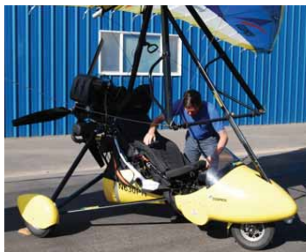
Figure 5-33. Installing the seats.
