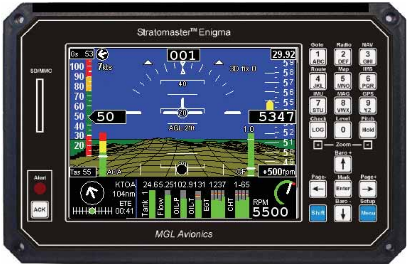
Figure 13-10. Digital panel with attitude indicator and direction indicator used on some WSC aircraft.
