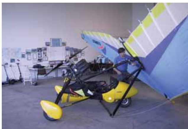
Figure 5-29. Attaching the mast to the wing after checking the POH for the proper hang point location.
