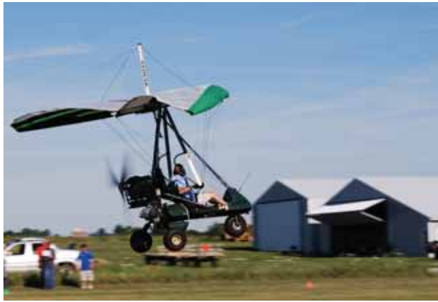
Figure 7-4. Initial takeoff grass strip with control bar pulled in slightly for a higher speed after liftoff in case of engine failure.
