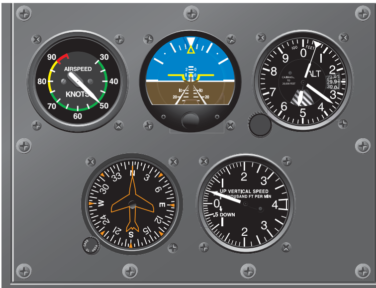
Figure 12-9. Classic instrument gauges for WSC aircraft.
