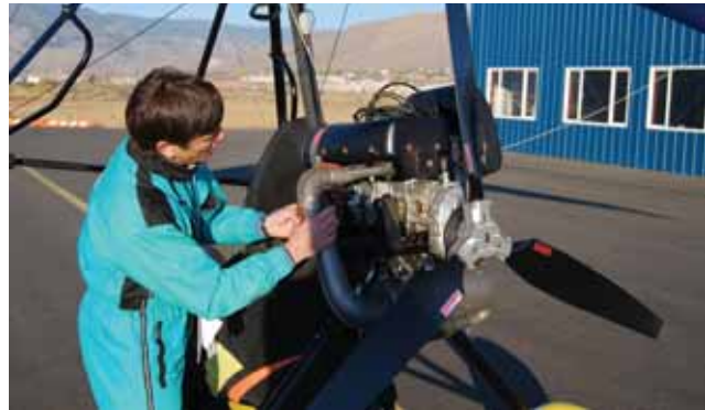
Figure 5-57. Inspecting the exhaust system by jiggling the outlet pipe and checking the springs.
