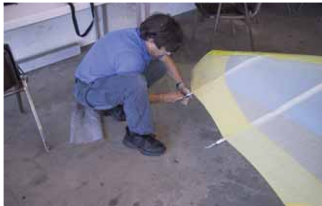
Figure 5-27. Installing the wing tip battens.
