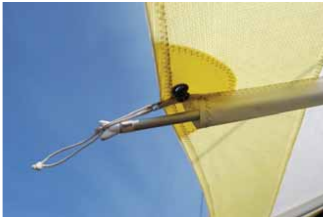
Figure 3-12. Trailing edge of the sail showing reinforcement panels, trailing edge line, and batten ties with attachment hardware.
