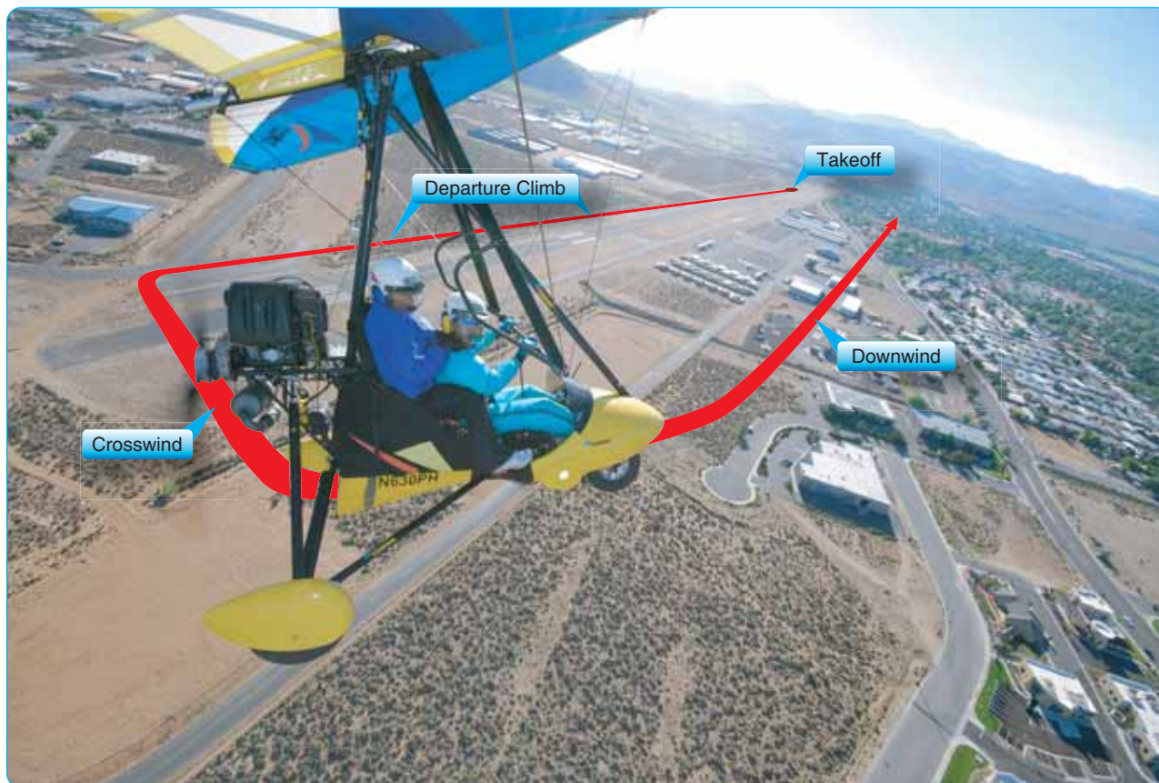
Figure 10-2. After takeoff and departure, turning from the crosswind to the downwind leg while climbing to pattern altitude.
