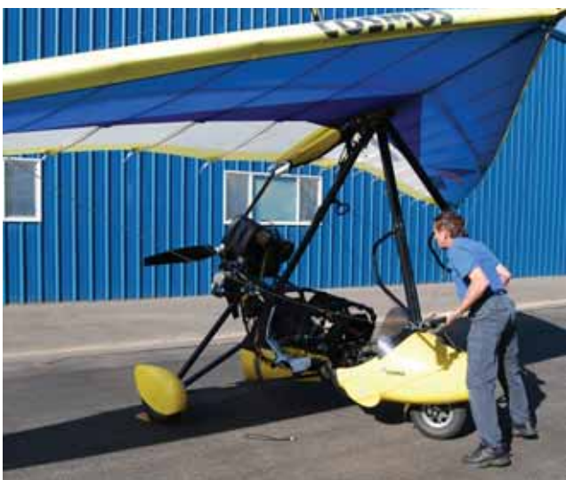
Figure 5-31. Lifting the wing up into position.
