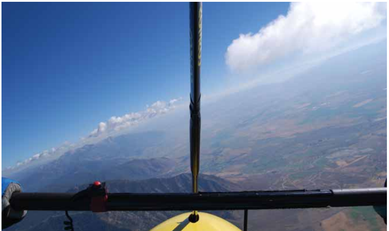
Figure 6-18. Pilot's visual reference of pitch and roll—continuing the shallow bank turn but raising the nose slightly with power application. Notice the how the front tube has moved across the horizon and the nose has raised slightly with additional power application to level flight.
