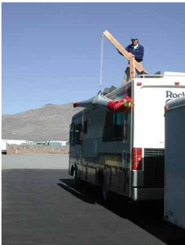
Figure 5-10. Crane used for one person to lift 110-pound wing on top of RV for transport.
