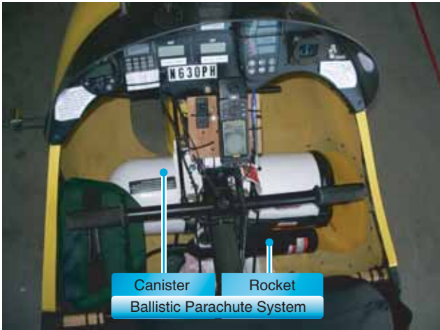
Figure 3-41. Located under the pilot's legs, the canister will blow through the break-away panel in the cowling.
