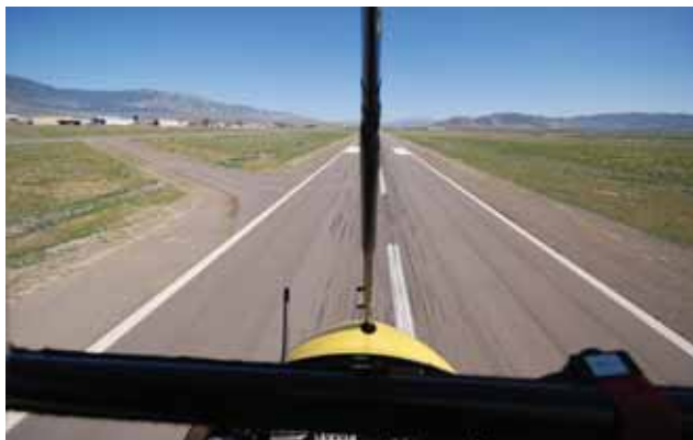
Figure 11-8. Starting the roundout by increasing angle of attack (AOA) slightly at about 10 to 15 feet above the runway.
