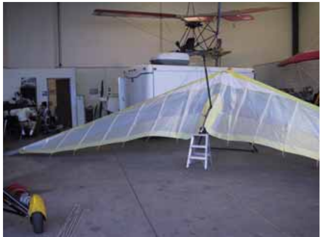
Figure 5-23. Wing ready to tension.
