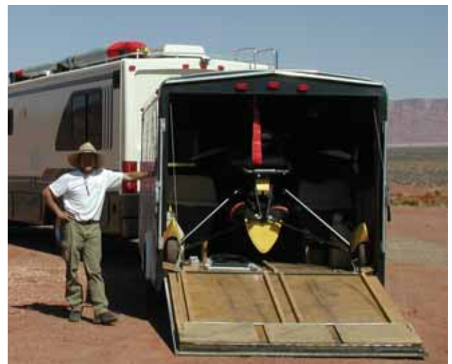
Figure 1-14. Wing folded and on top of a recreational vehicle with the carriage in a trailer.
