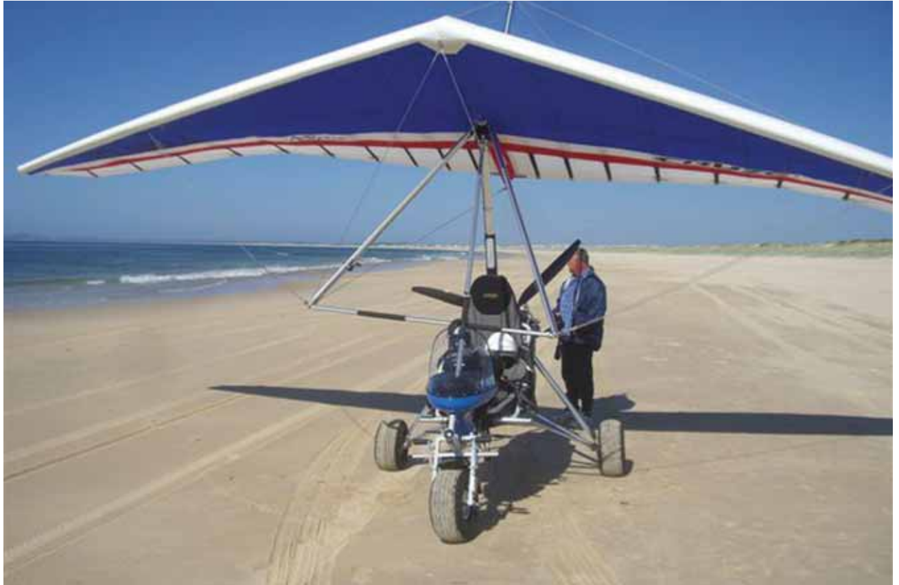
Figure 7-12. Example of a WSC aircraft designed with a wide low-pressure front wheel for soft field operation.
