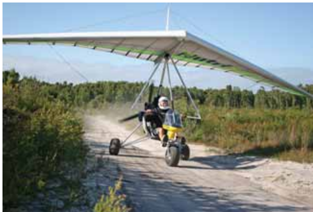
Figure 3-38. WSC aircraft with large tundra tires for soft or rough field operations.
