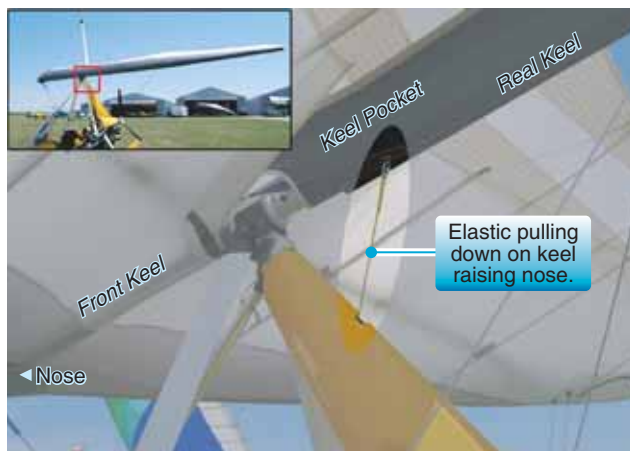
Figure 3-24. More tension on elastic pulling down on the rear of the wing keel reduces the trim speed and is controlled by the pilot in flight.
