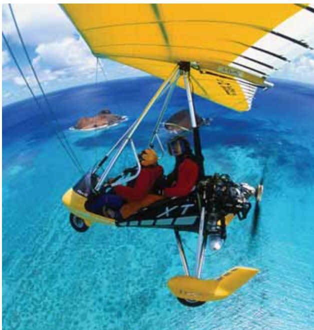
Figure 2-34. Wheel fins for carriage yaw stability.
