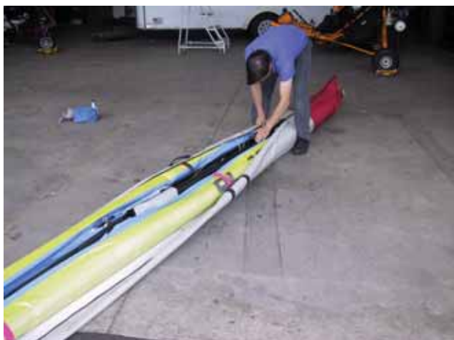
Figure 5-38. Carefully zipping bag with minimum stress by tucking in wires and organizing components.
