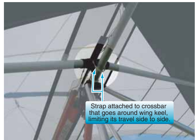
Figure 3-21. Crossbar travel limiter.
