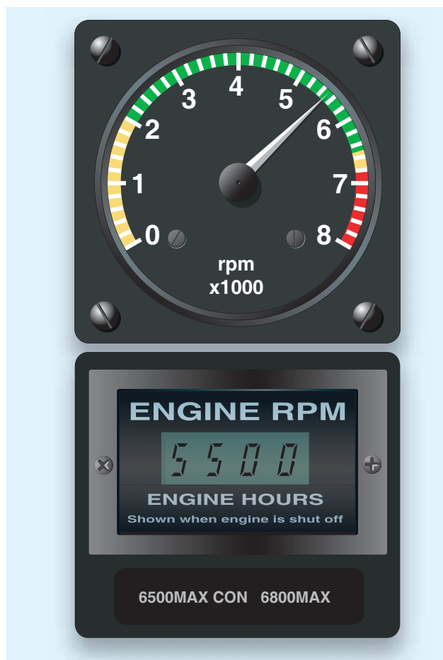
Figure 4-9. Engine rpm is indicated on the analog gauge (top) and the digital gauge (bottom).
