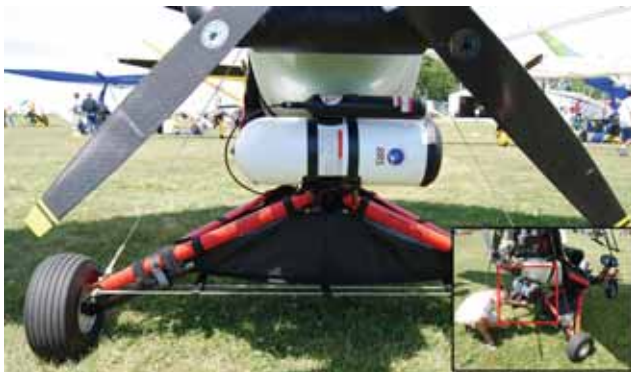
Figure 3-42. Canister mounted under engine.
