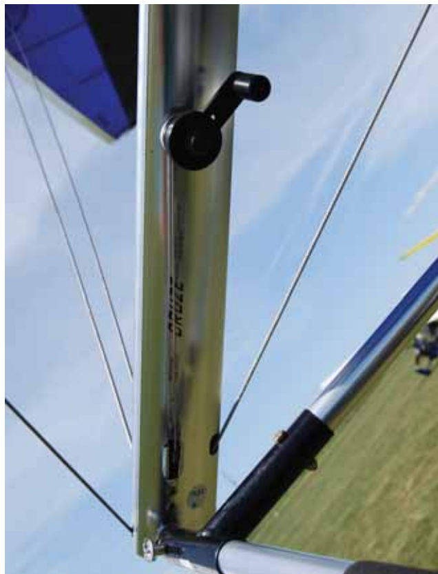
Figure 3-22. A crank on the downtube of the control bar that adjusts the trailing edge reflex during flight.
