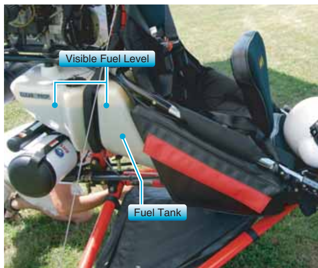
Figure 3-50. Fuel tank with visible fuel quantity.
