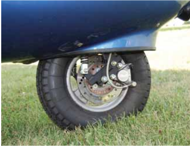
Figure 3-31. Hydraulic disk brake system.
