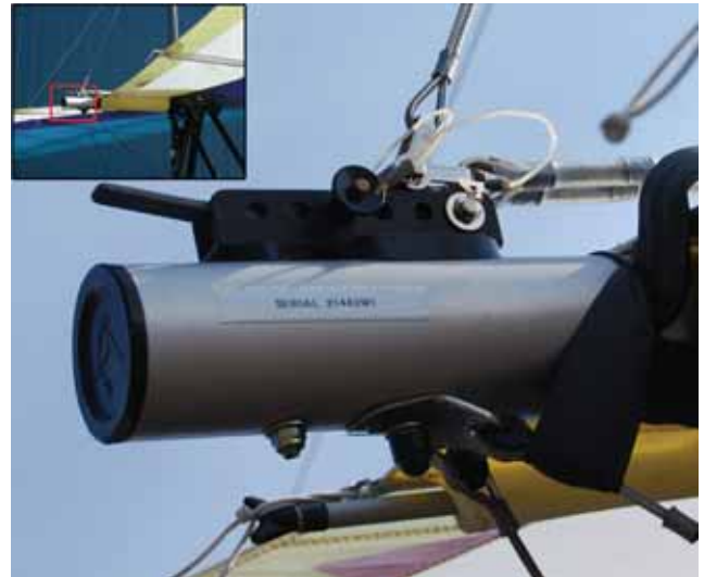
Figure 3-14. Crossbar tensioning junction attachment example.
