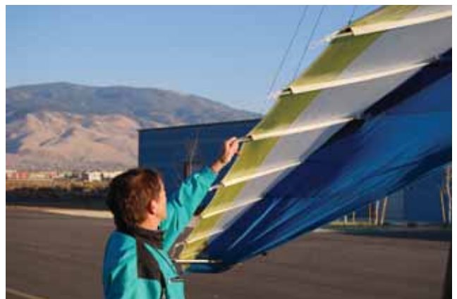
Figure 5-46. Inspecting the trailing edge of the wing.
