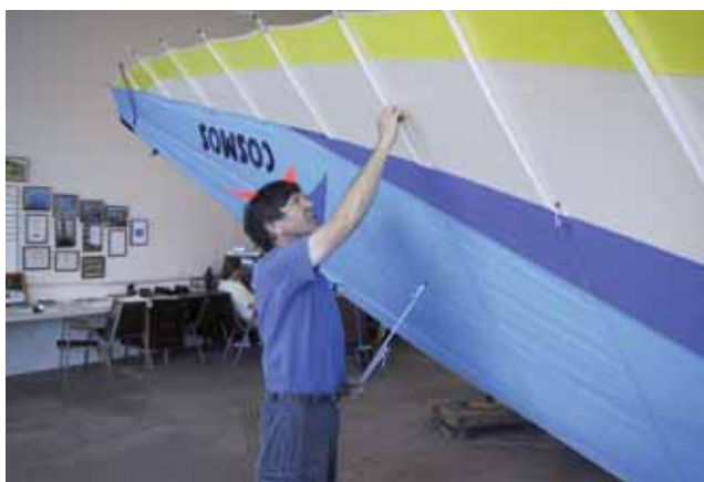
Figure 5-28. Installing the lower surface battens.
