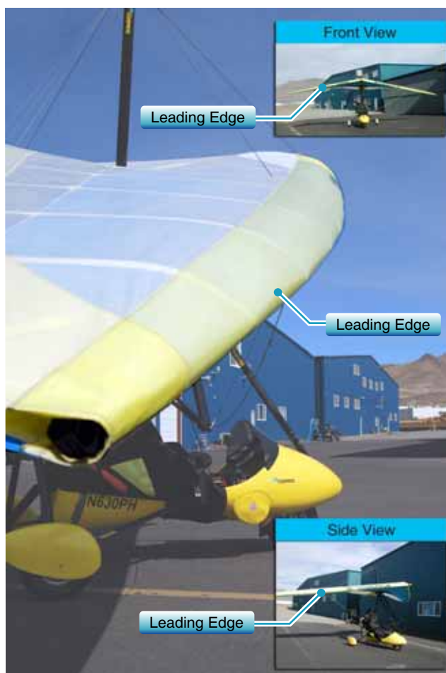
Figure 3-11. Curved leading edge sail design.
