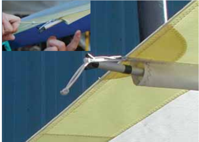
Figure 5-22. Attaching double pull batten (inset). Batten secured into batten pocket.
