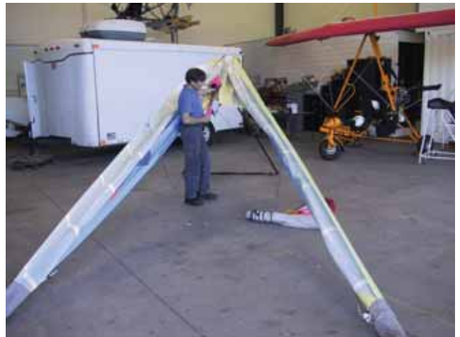
Figure 5-17. Wings spread slightly to raise the kingpost.
