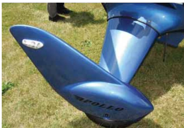
Figure 3-37. Solid flexible main landing gear that is streamlined.
