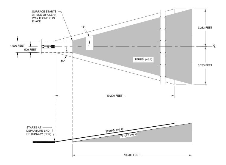
Figure A2-3. Departure surface for Instrument Runways TERPS (40:1)
