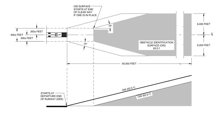
Figure A2-4. One-Engine Inoperative (OEI) Obstacle Identification Surface (62.5:1)
