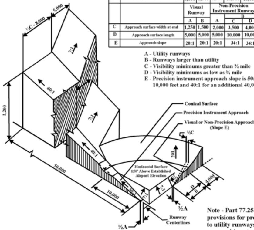
Note - Part 77.25 does not make provisions for precision approaches to utility runways. In these situations, use precision standards for other than utility runways to develop the primary, approach, and transition surfaces.
