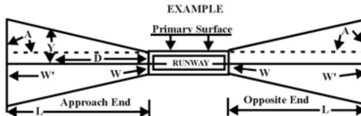
**Sample Use Problem:** Proposed structure would be located by measurement to be 20,000 feet from the end of the primary surface and 3,400 feet at 90° from the extended centerline of a precision runway (refer to Section 77.21(b) for relation of primary surface to end of runway). To determine whether it would fall within the approach surface of that runway, apply the following formula:
