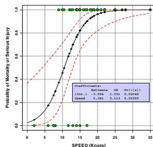
Figure 1. Fitted logistic regression showing the relationship between serious injury and vessel speed. (Green dots are observed, black diamonds are predicted and red-dashed lines are the 95% CI about the individual predicted values.
