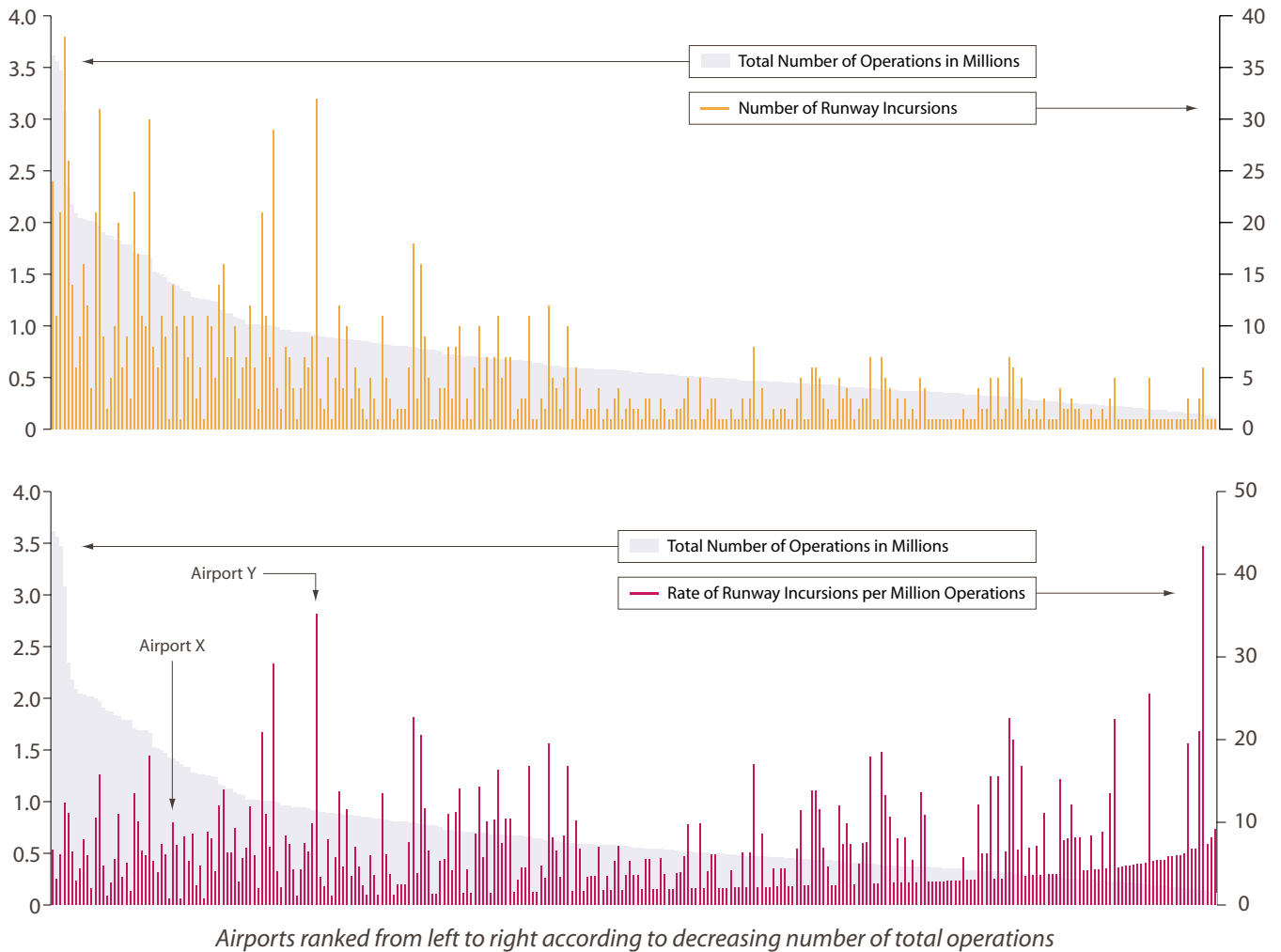
Figure 3. The relationship between traffic volume and runway incursion number and rate at U.S. Towered Airports (CY 1998 through CY 2001)
