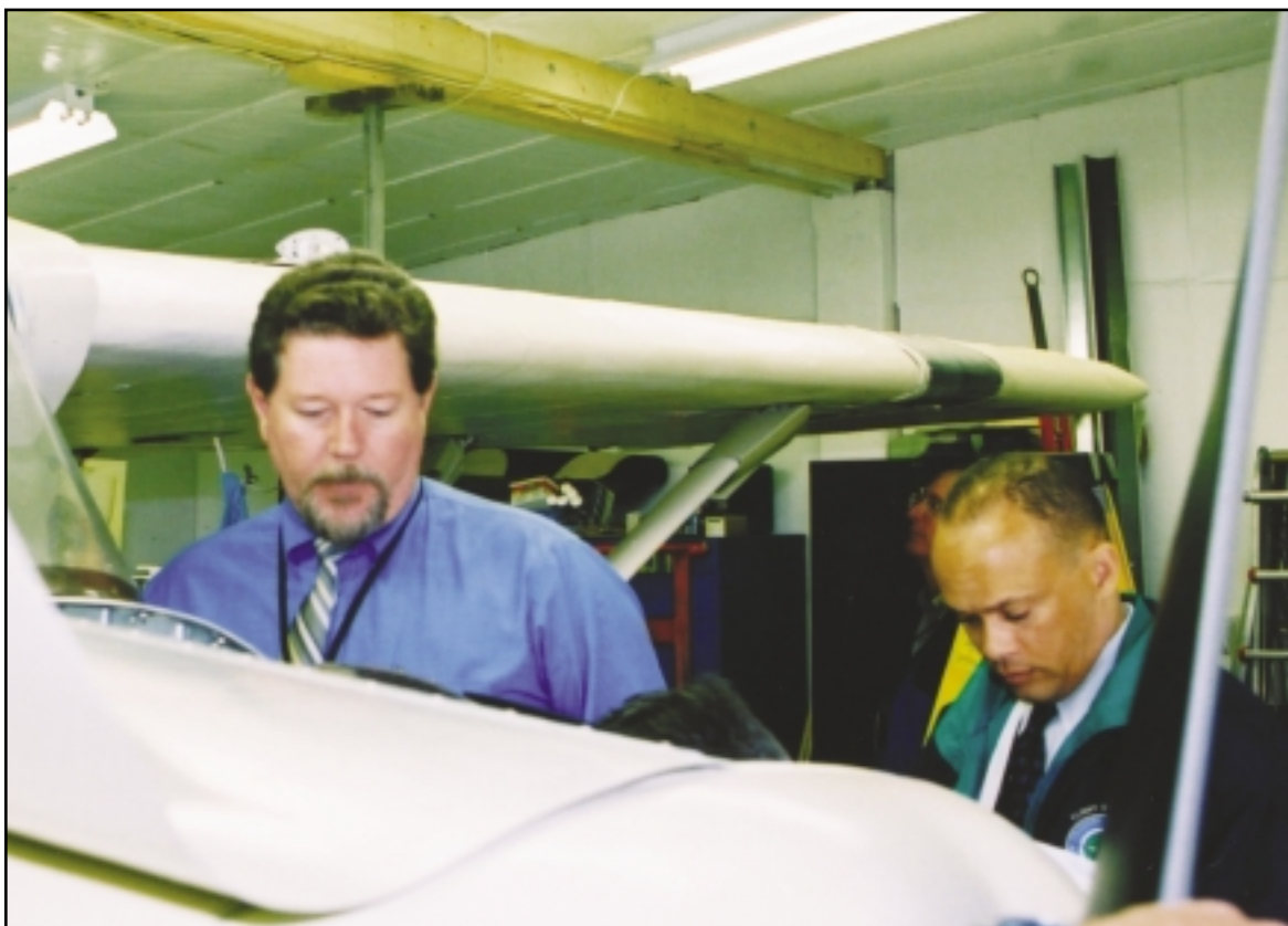
FAA inspectors Robert Nolan (l) and Troy Lawson check for proper installation, correct hardware, security, safety wire, any chaffing or pinch points, and any interference problems as part of their inspection.
