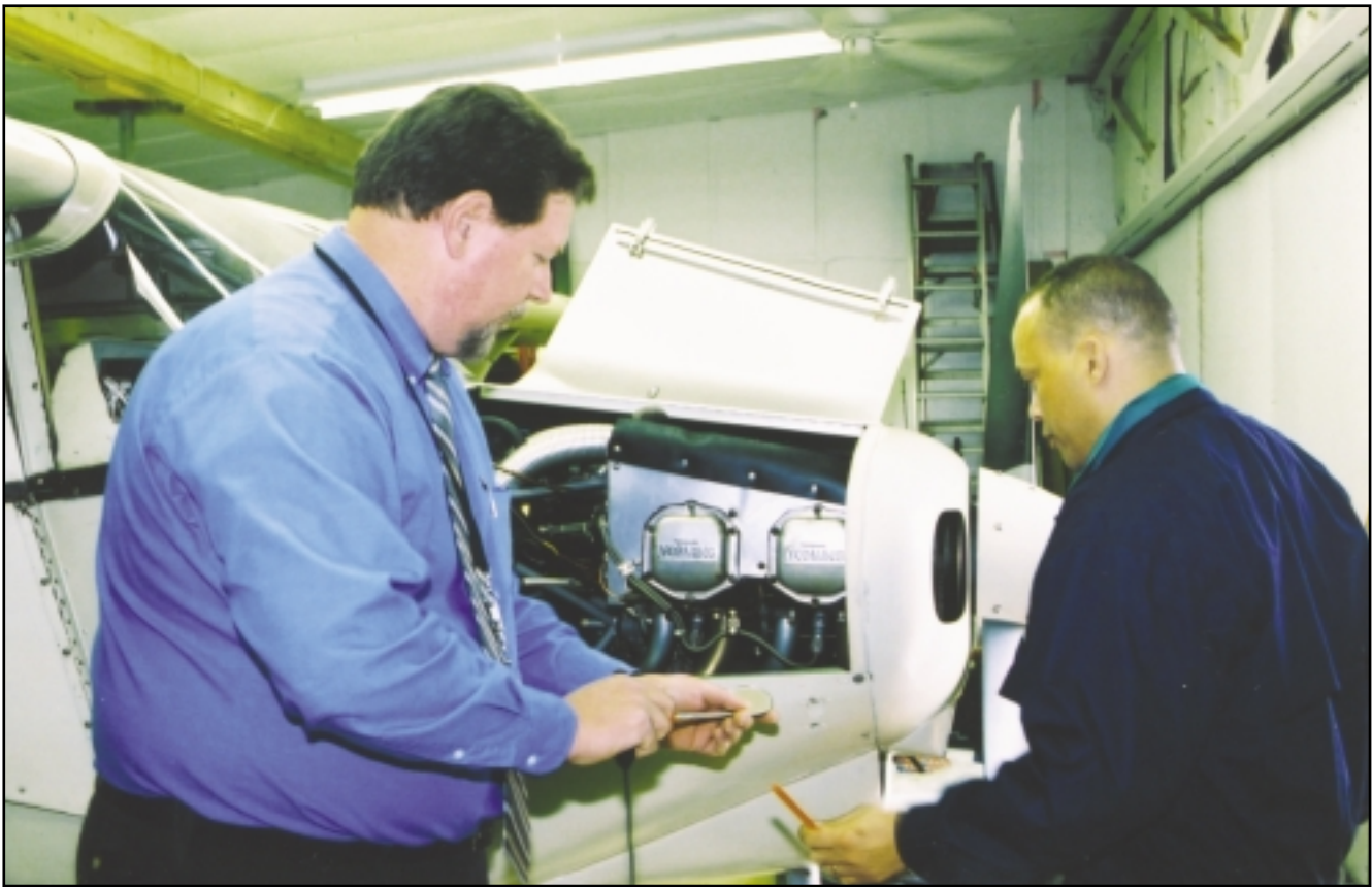
FAA airworthiness inspectors Robert Nolan (l) and Troy Lawson prepare to inspect the engine compartment of the Orphan. With new electrical wiring, new fuel and oil lines, and a new alternator replacing the original generator, the inspectors want to make sure all the hardware was properly installed.
