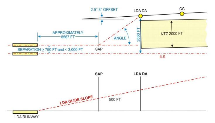
**SAP.** The SAP is a design point along the extended centerline of the intended landing runway on the glide slope at 500 ft above the touchdown zone elevation. It is used to verify a sufficient distance is provided for the visual maneuver after the LDA PRM DA to permit the pilots to conform to approved, stabilized approach criteria.
