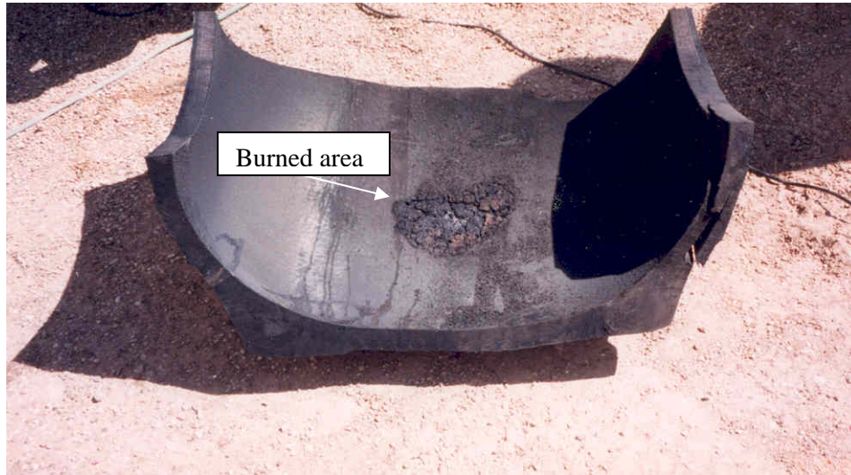
Figure 1 – Burned Area of a Mine Vehicle Tire that Exploded
