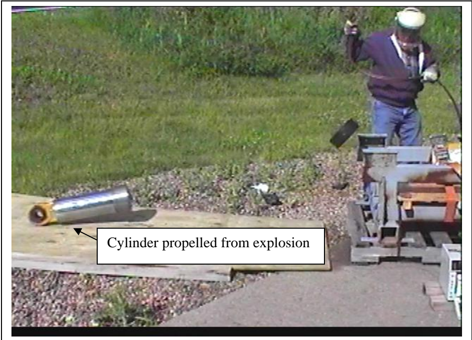
Figure 4 – Empirical Test Illustrating an Explosion in an Equipment Cylinder
