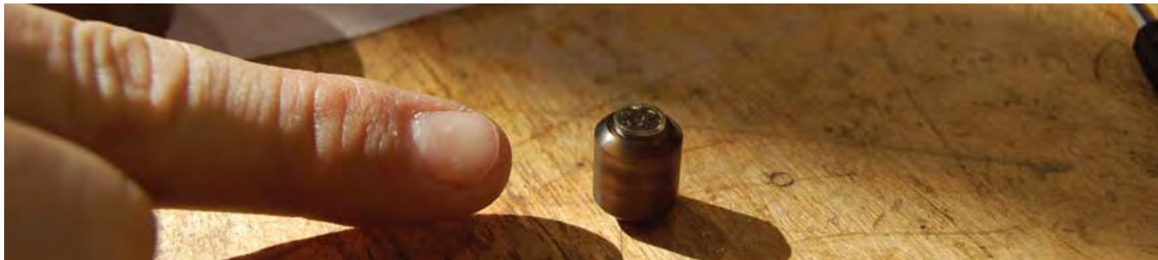
Once assembled, the diamond anvil cell is no bigger than a fingertip.
