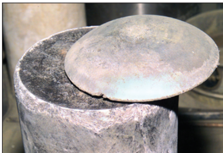
From top to bottom: Plutonium dioxide is the feed material for the MCDOR process. After the reaction is complete, the melt settles and cools, forming a plutonium button at the bottom of the crucible and a calcium chloride salt cake above it. The crucible is broken away and the plutonium button is mechanically separated from the salt cake. In the lower photo the plutonium button is pictured on top of the salt cake.
