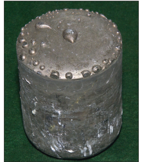
This plutonium ingot, produced by coalescence, will be the feed material for the electrorefining process.
