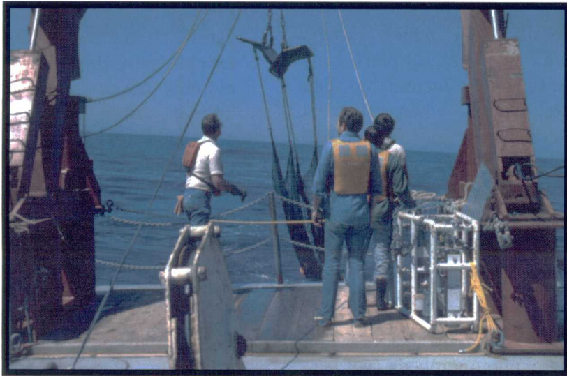
A bottom trawl coming on board the research vessel as the deep-sea camera system awaits its turn to photograph the same depth zone.
