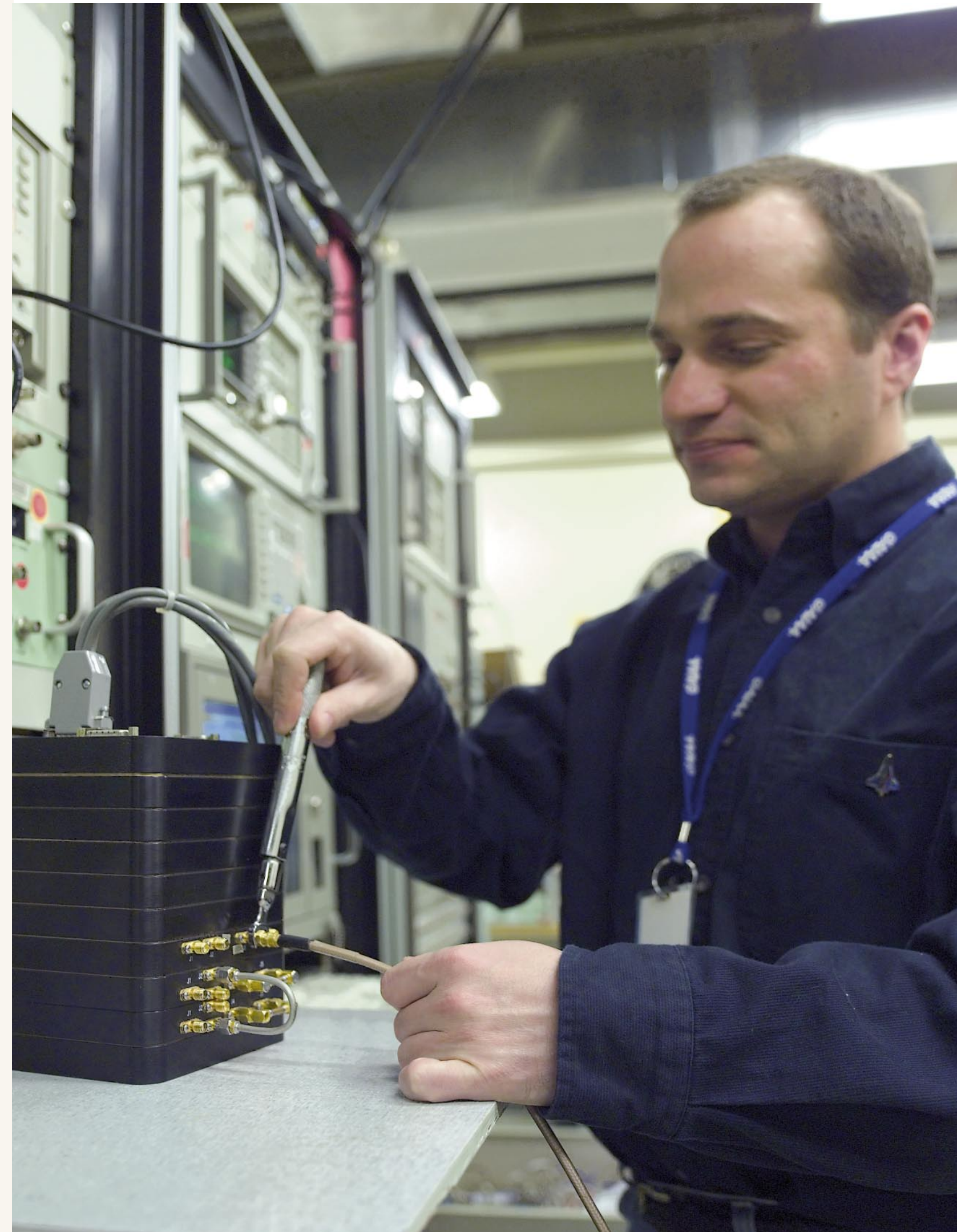
Goddard researchers flew this experiment — the Communications and Navigation Demonstration on Shuttle (CANDOS) — to test the integrated communications and navigational functions of a new modular multiband, multi-channel transceiver developed by Goddard and ITT Industries.
