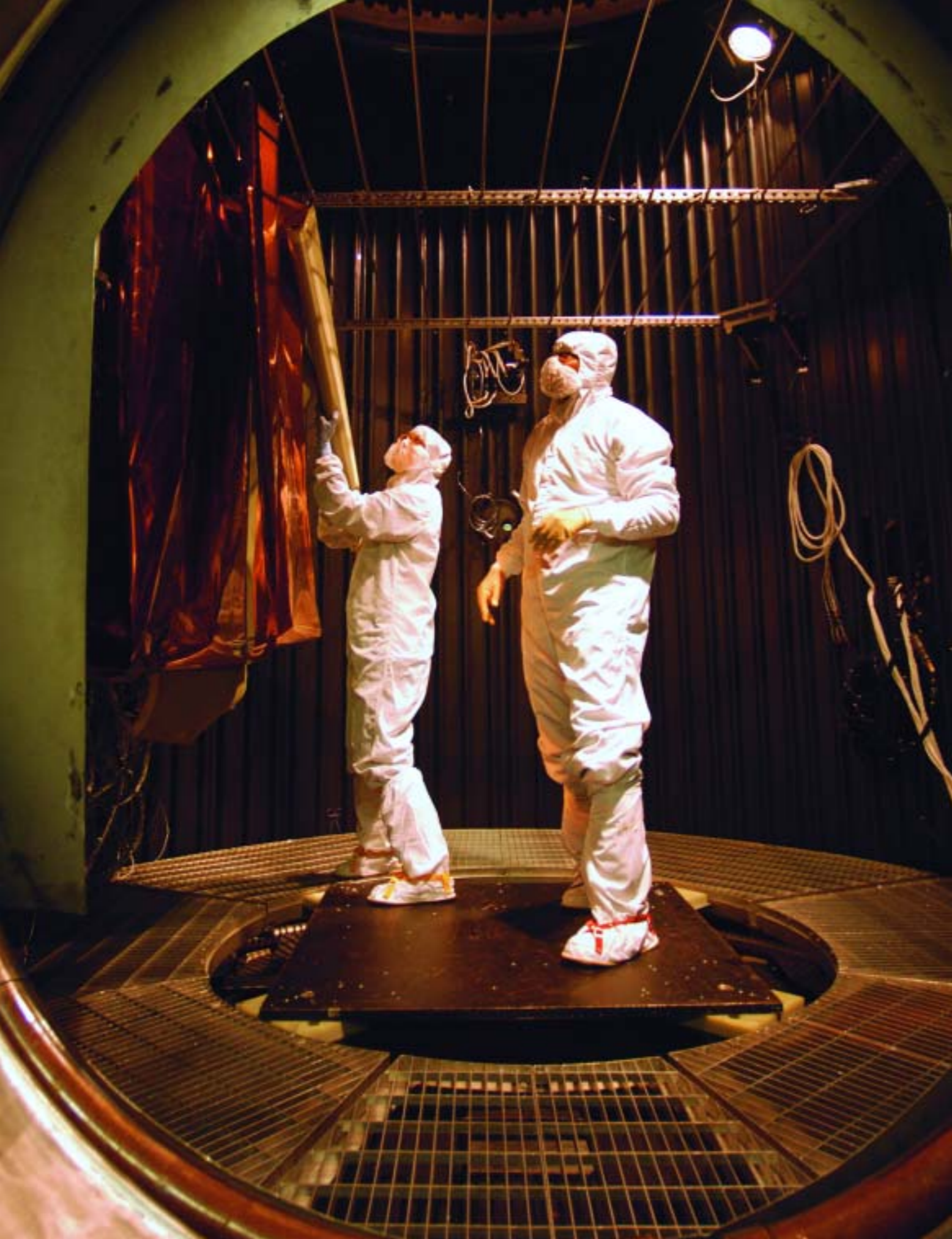
NASA technicians remove Germanium black Kapton film after testing in one of Goddard's many vacuum chambers.
