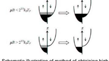
Schematic illustration of method of obtaining high spin polarizations in degenerate Fermi fluids.
