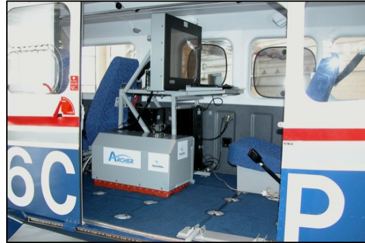
ARCHER system installed with custom-designed rack and protective hood in the Gippsland GA-8 Airvan
