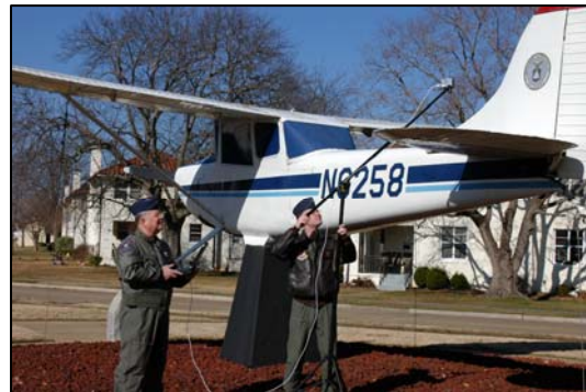
HSI operators collect the spectral signature of an aircraft on static display outside the CAP National Headquarters building at Maxwell AFB, Ala. The signature is then entered into the ARCHER airborne system and used in a test to determine if the HSI equipment will pinpoint the static display plane from the air.
