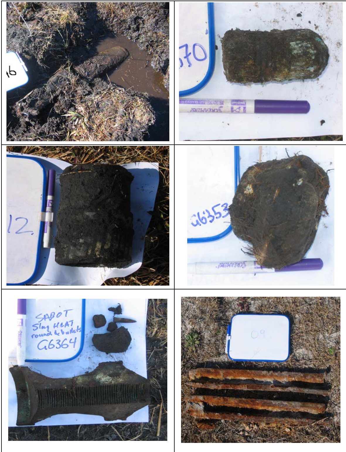
Figure 6. Examples of ground-truth data collected on Range G6, including a 120-mm HEAT Rocket (top left), 40-mm practice grenade (top right), adapter (center left), adapter part (center right), part of a discarding sabot and other OE scrap (bottom left), and four steel pipes (bottom right).
