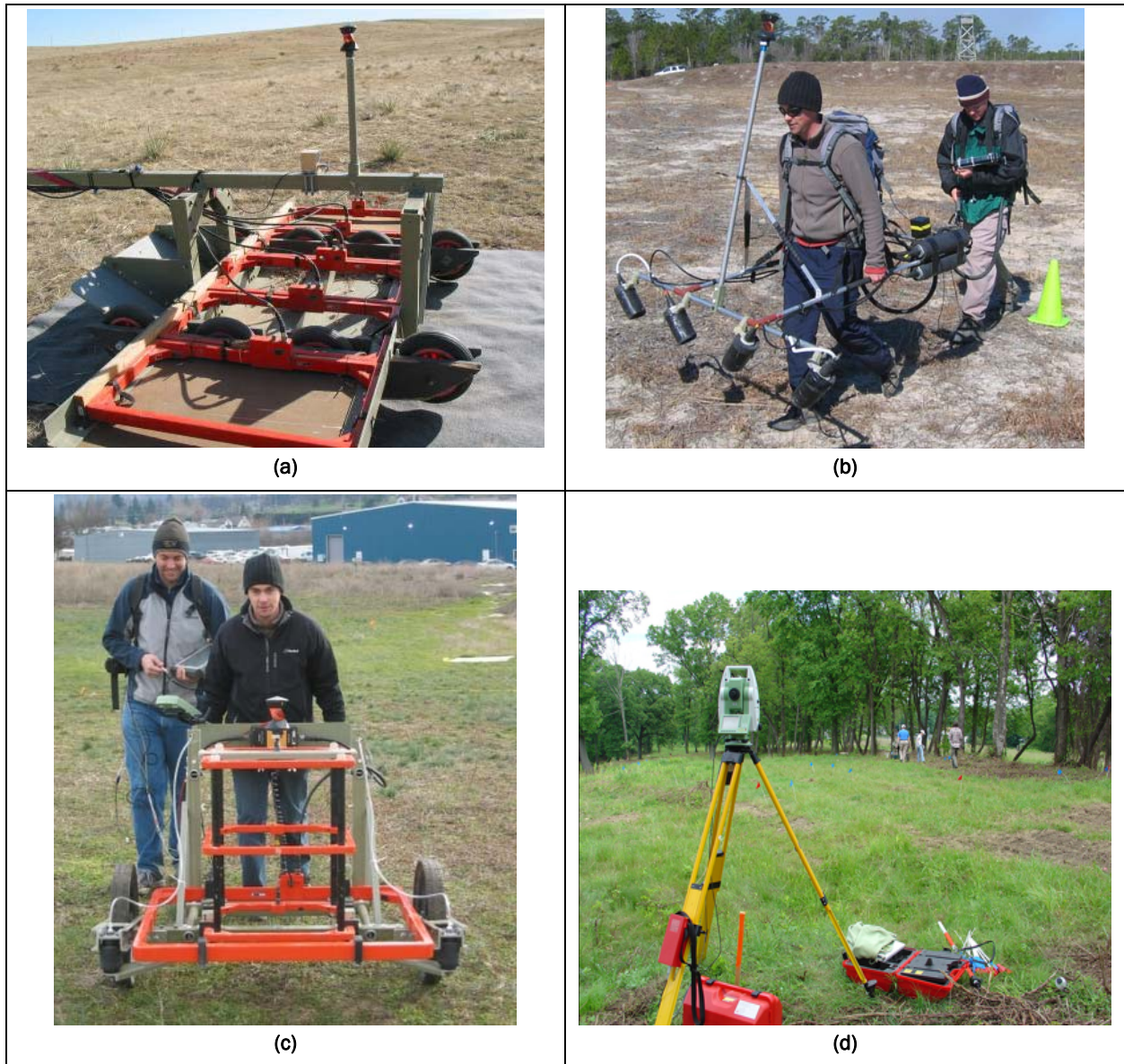
Figure 1. Discrimination mode platforms used to collect data at Camp Lejeune: (a) Geonics EM-61 MKII towed array; (b) quad-sensor magnetometer array; (c) Geonics EM-63; (d) Leica RTS.
