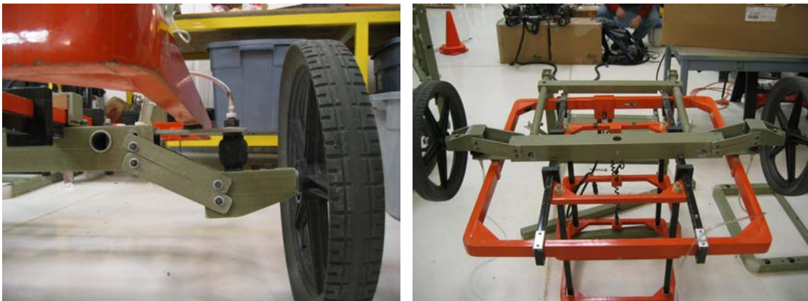
Figure 19. Modified EM-63 cart, which is lower to the ground and has an air suspension system. The left-hand image provides a close-up of the air-suspension, while the right-hand image shows the cart upside down.
