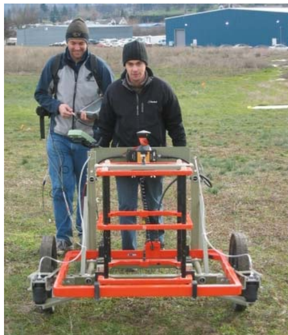
Figure 20. Modified EM-63 cart collecting discrimination mode data at the Ashland test site.
