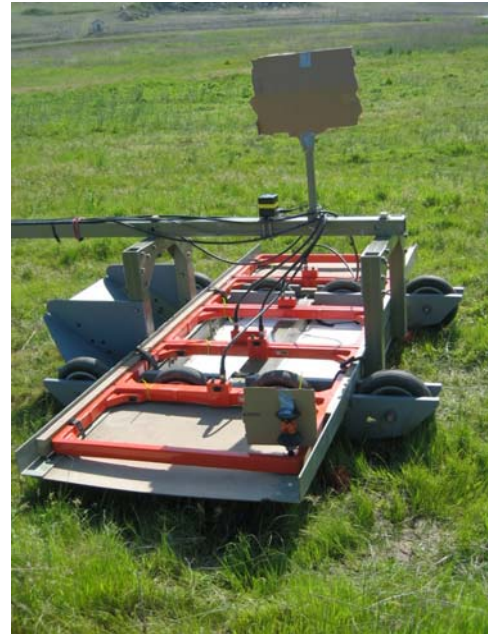
Figure 8. Two-RTS test of the positional accuracy of the towed array. Rectangular pieces of card-board were used to shield each prism from the other RTS base-station. At the end of each line, the card-board was moved to the other side of the each prism so that the same gun tracked the same prism.
