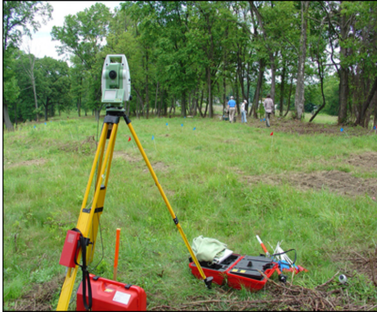
Figure 1. Sky Research utilizes the Leica RTS TPS1206 laser positioning system. This device is set up over a known point and tracks a prism attached to the geophysical survey equipment. RTS technology out-performs GPS in terms of accuracy, sampling rate, and operational ease of use.
