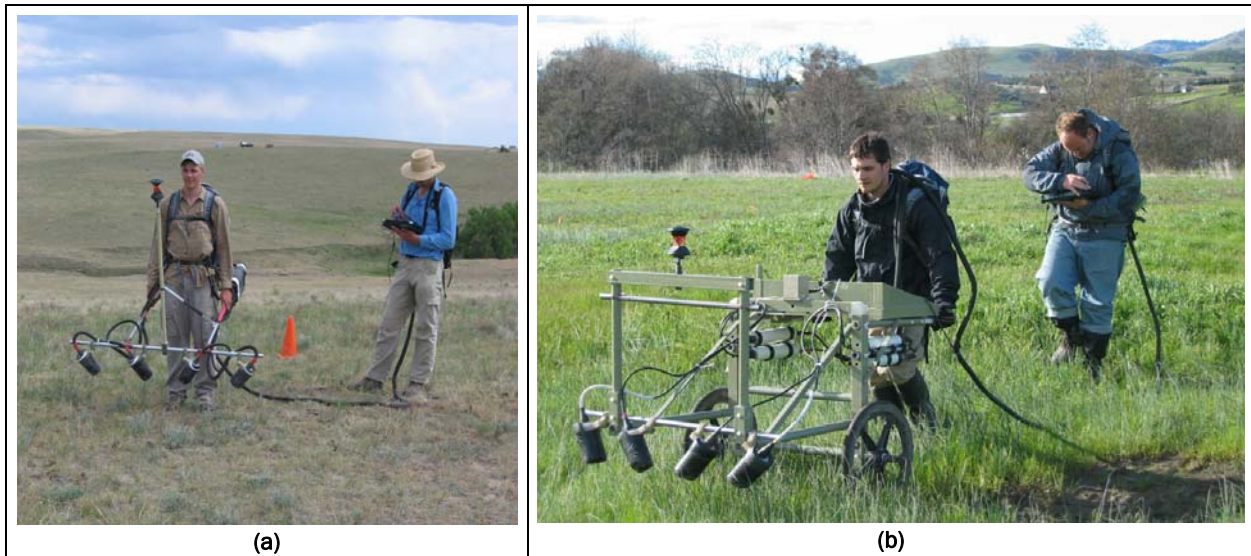
Figure 26. Man-portable quad-sensor array (left) and cart-based magnetometer systems developed as part of this project. For the gradient configuration, the same cart was used with the upper sensors 50 cm above the lower ones.
